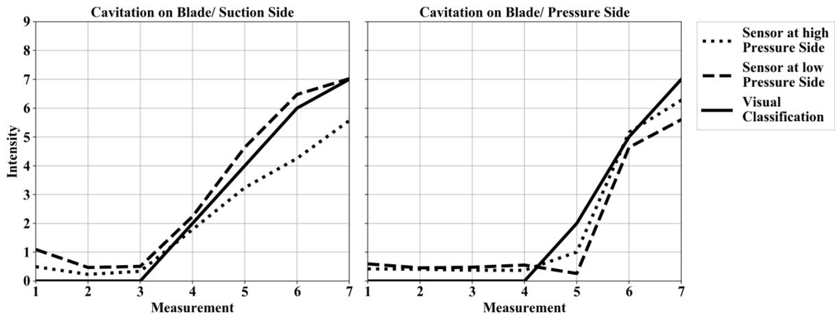
Figure 4: Estimated vs. real Intensity
