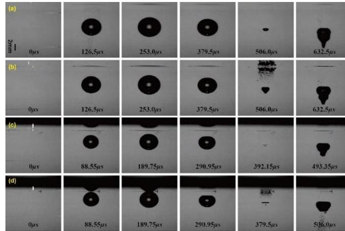
Fig. 2. Laser-induced bubble behaviors near a flat free surface with different  $h/R_{max}$ . (a)  $h/R_{max}=2.261$ ,  $T_c/T_c'=0.916$ ; (b)  $h/R_{max}=1.932$ ,  $T_c/T_c'=0.904$ ; (c)  $h/R_{max}=1.432$ ,  $T_c/T_c'=0.862$ ; (d)  $h/R_{max}=1.027$ ,  $T_c/T_c'=0.846$ . The scale bar is only valid on the vertical direction due to the image distortion from the cylindrical water flask.
