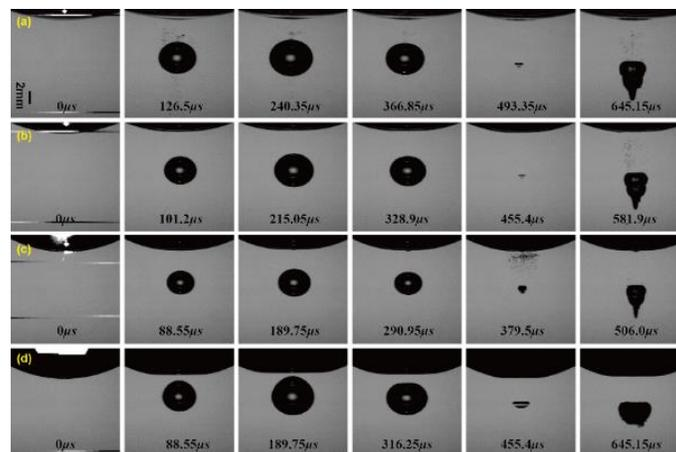
Fig. 3. Laser-induced bubble behaviors near a convex free surface. (a)  $h/R_{max}=1.977$ ,  $r_s/R_{max}=8.292$ ,  $T_c/T_c'=0.924$ ; (b)  $h/R_{max}=2.125$ ,  $r_s/R_{max}=5.458$ ,  $T_c/T_c'=0.938$ ; (c)  $h/R_{max}=2.152$ ,  $r_s/R_{max}=5.710$ ,  $T_c/T_c'=0.948$ ; (d)  $h/R_{max}=0.977$ ,  $r_s/R_{max}=4.304$ ,  $T_c/T_c'=0.897$ . The scale bar is only valid on the vertical direction due to the image distortion from the cylindrical water flask.
