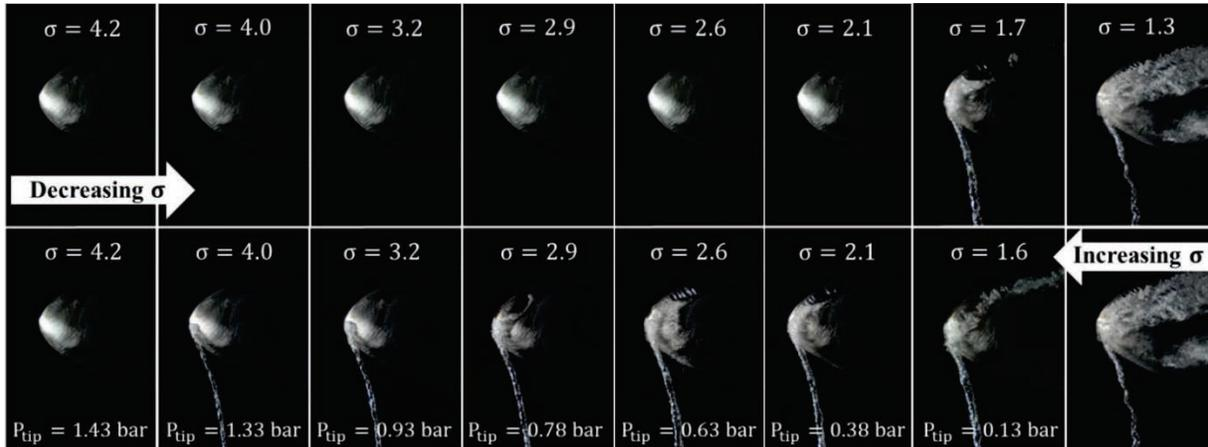
Figure 1: Hysteresis in TVC inception and desinence at  $V_\infty = 10$  m/s,  $\alpha = 12^\circ$ , and 100 % of O<sub>2</sub> saturation
