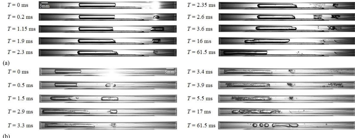
Fig.3 Gas removal by an oscillating bubble in a rigid tube. (a. The whole liquid moves towards left. b. The whole liquid moves towards right.)
