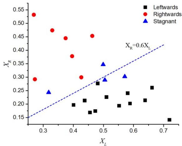
Fig.4 Flow direction after the collapse of the spark-generated bubble
