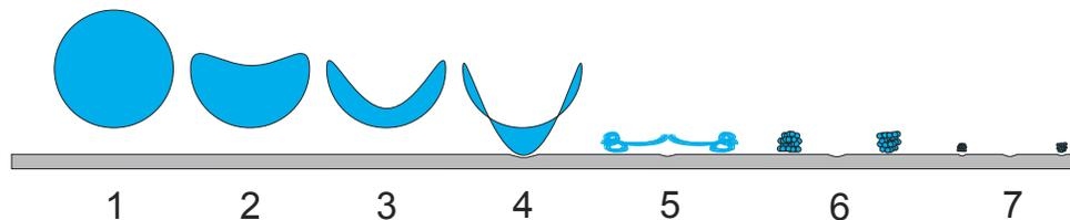
Figure 1: Two possible mechanisms of cavitation erosion.
