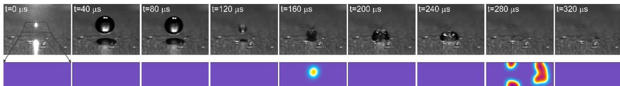
Fig. 6: Bubble and damage for collapse far away from the wall ( $\gamma=1.7$ )
