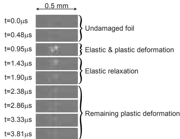
Fig. 8: Damage evolution recorded at 2.1 Mfps.
