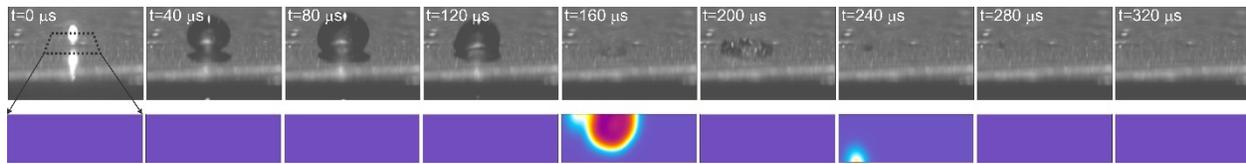
Fig. 7: Bubble and damage appearance in the presence of shear flow ( $\gamma=1.0$ ,  $v=2.5$  m/s)
