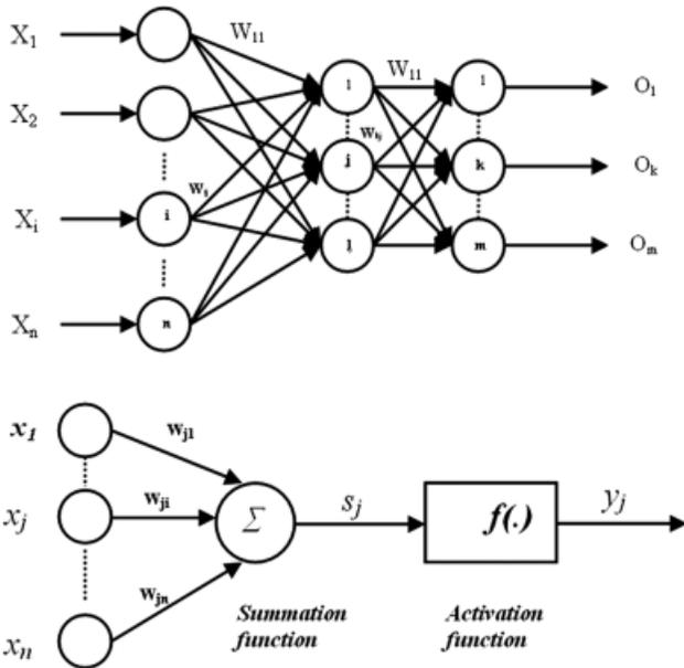
Figure 1 | Typical three-layer feed-forward artificial neural network.
