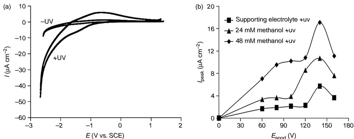
**Figure 3** | (a) Cyclic voltammograms in supporting electrolyte (0.1M NaOH) on the electrode anodized at 140V in the dark and under illumination, at a scan rate of 100 mV/s and (b)  $I_{\text{peak}}$  vs. Anodization voltage (V) under illumination.
