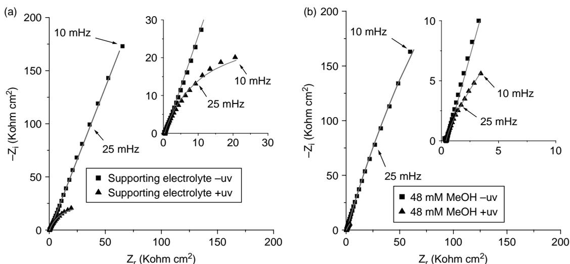
Figure 5 | Nyquist diagrams ( $-Z_{im}$  vs.  $Z_{re}$ ) for the Ti/TiO<sub>2</sub> electrode prepared at 140 V, (a) in 0.1 M NaOH, (b) in the presence of 48 Mm of methanol.
