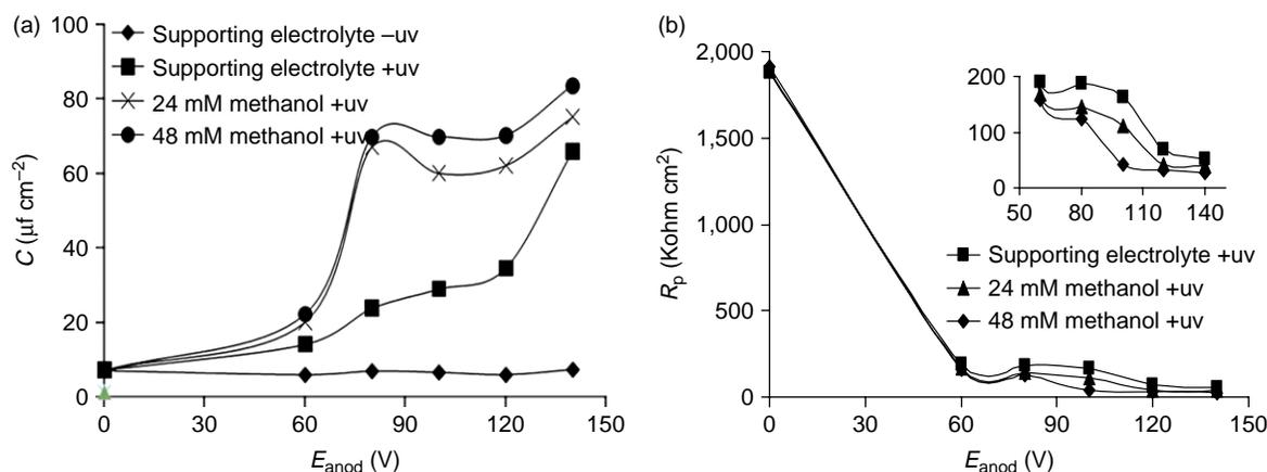
Figure 6 | EIS fitting parameters function of anodization potential, (a) capacity, (b) polarisation resistance ( $R_p$ ).
