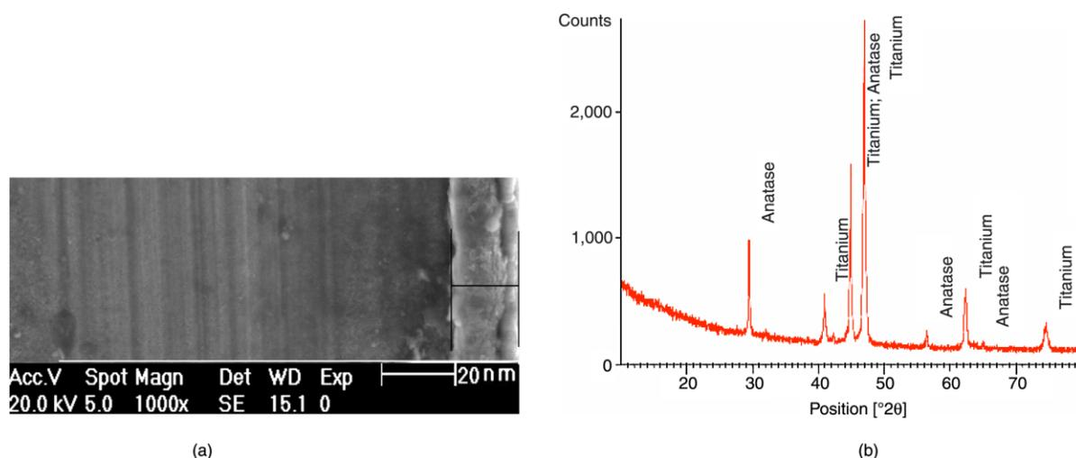
Figure 1 | TiO<sub>2</sub> film (a) SEM observation ( $E_{\text{anod}}$  120 V), (b) XRD spectrum ( $E_{\text{anod}}$  140 V).
