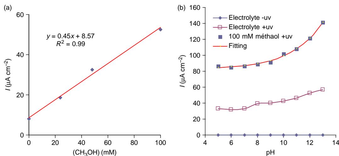
**Figure 8** | (a) Photocurrent vs. methanol concentration, pH = 13, (b) photocurrent of the TiO<sub>2</sub> electrode at different pH values both with and without illumination and fitted curve,  $E = 1\text{ V/SCE}$ , 100 mM methanol.
