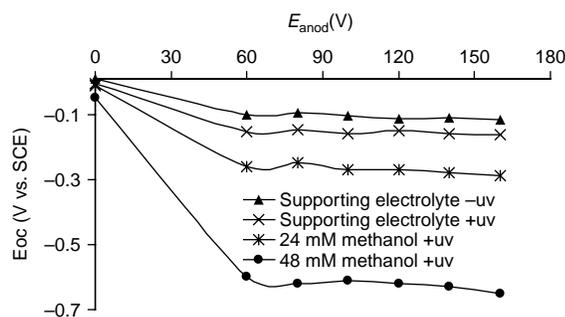
**Figure 2** | Open-circuit potential vs. anodization voltage ( $E_{\text{anod}}$ ) in 0.1 M NaOH, in the dark (−UV) and under illumination (+UV) and in the presence of 24 and 48 mM of methanol.
