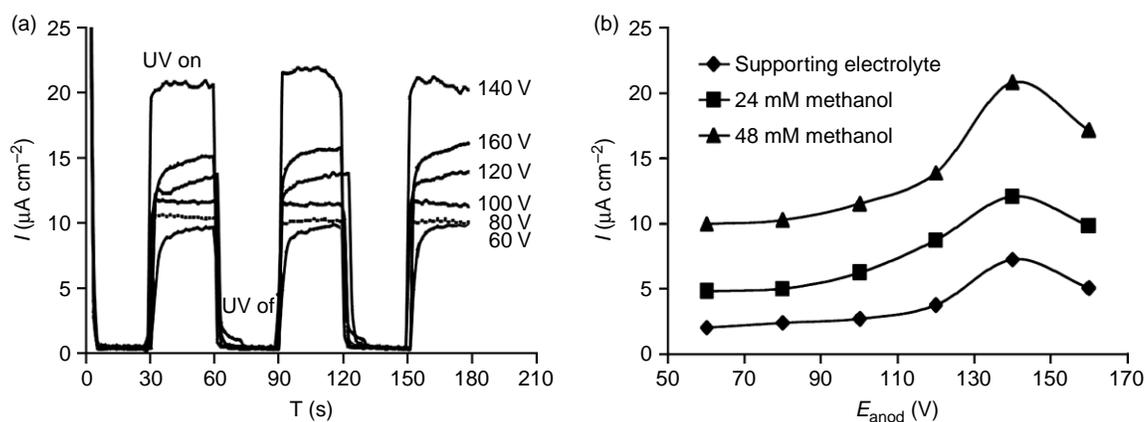
**Figure 4** | (a) Photocurrent-time characteristics of different electrodes measured at  $E = 1\text{ V/SCE}$  and (b) photocurrent vs. anodization voltage ( $E_{\text{anod}}$ ).
