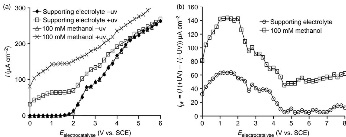
Figure 7 | (a) Current registered vs. electrocatalytic potential (b) calculated photocurrent vs. electrocatalytic potential, electrode anodized at 140 V, degradation time 30 min and pH = 13.
