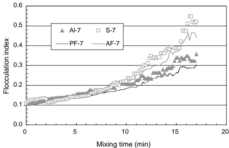
**Figure 3** Effect of different chemical addition sequences (aluminium chloride dosage at 7 mg/L and the cationic polymer at 0.07 mg/L)
