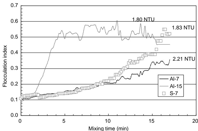
Figure 1 Comparison of single use of aluminium chloride with use of dual coagulants (aluminium chloride at 7, 15 mg/L and the cationic polymer at 0.07 mg/L)
