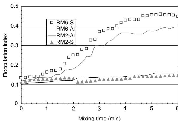
**Figure 2** Rapid mixing effect (rapid mixing for 2 min and 6 min at aluminium chloride dosage at 7 mg/L and the cationic polymer at 0.07 mg/L)
