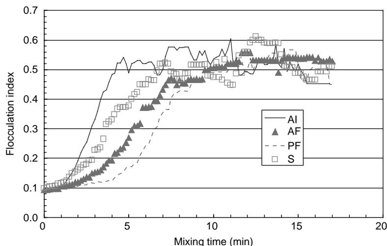
**Figure 4** Effect of different chemical addition sequences (aluminium chloride dosage at 15 mg/L and the cationic polymer at 0.07 mg/L)
