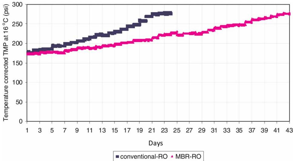
Figure 4 | Run 2 fouling rate of RO systems.
