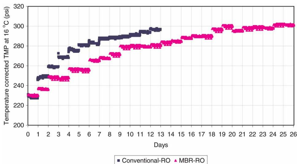
Figure 3 | Run 1 fouling rate of RO systems.
