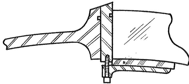
Fig. 15 Recommended design changes for top hatch (compare with Fig. 2a)
