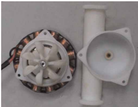
Figure 2 | The pipe flow generator in this study.
