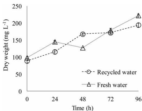
**Figure 4** | Microalgae growth over time in two independent photobioreactors fed with swine wastewater digestate effluent diluted with either fresh tap water or recycled supernatant water from coagulation/flocculation process. Bars represent standard error from the mean.
