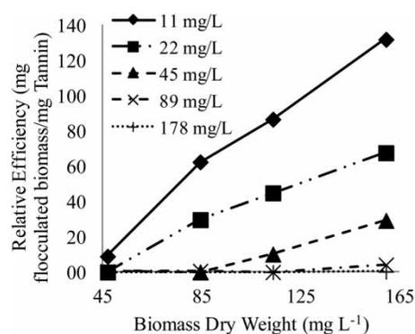
**Figure 2** | Effect of different TAN dosages on coagulation/flocculation recovery efficacy (mg flocculated *Chlorella vulgaris* biomass per mg TAN).
