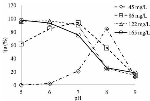
**Figure 3** | Effect of pH on coagulation/flocculation recovery efficiencies ( $\eta_a$ ) for different concentrations of *Chlorella vulgaris* biomass. Coagulant TAN tested at  $22 \text{ mg L}^{-1}$ . Bars represent standard error from the mean.
