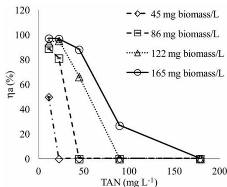
**Figure 1** | Effect of TAN dosages on the coagulation/flocculation recovery efficiency ( $\eta_a$ ) as a function of *Chlorella vulgaris* biomass concentrations (45, 86, 122 and 165 mg L<sup>-1</sup> DW). Experiments conducted at pH 7. Bars represent standard errors from the mean.
