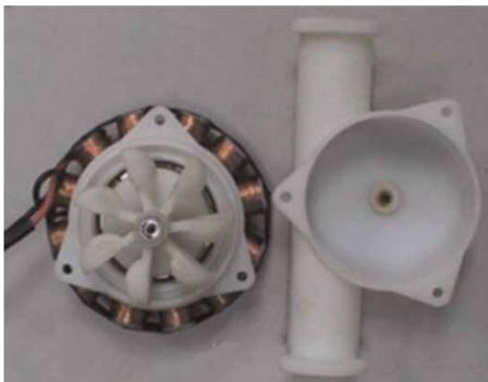
Figure 2 | The pipe flow generator in this study.
