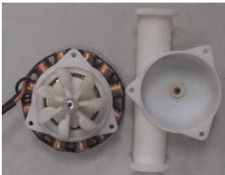
Figure 2 | The pipe flow generator in this study.
