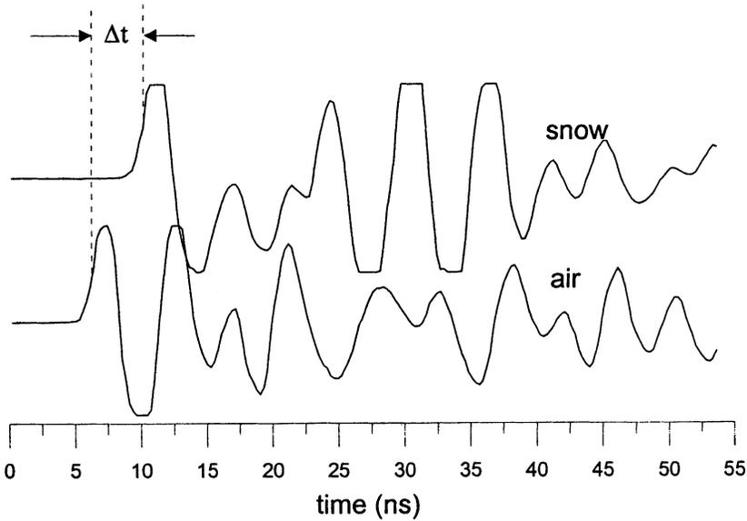
Fig. 2. Example of measured trace in snow (top) and in air (bottom). Only the first arrivals are considered. The position of the time scale is arbitrary since only the difference in arrival time ( $\Delta t$ ), *i.e.* the time delay due to the wet snow, is of importance.  $\Delta t$  is in this example 3.9 ns.
