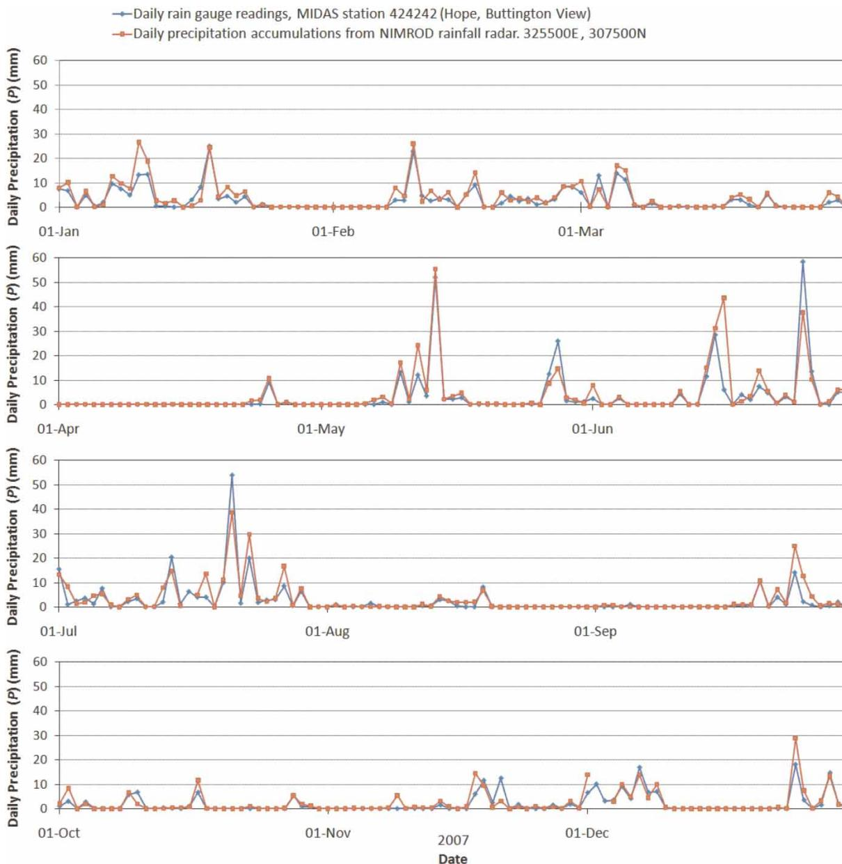
**Figure 2** | Daily precipitation for 2007 from MIDAS station 424242 (Hope, Buttington View 325900E, 307400N) (readings taken at 09:00 UTC) ( $P_{RG}$ ) and NIMROD radar data daily accumulations (09:00 UTC to 08:55 UTC) from 1 km grid square centred on 325500E, 307500N ( $P_N$ ). NIMROD data were missing for 16 July, 2 December and 3 December 2007. Data from [BADC \(2010b\)](#).
