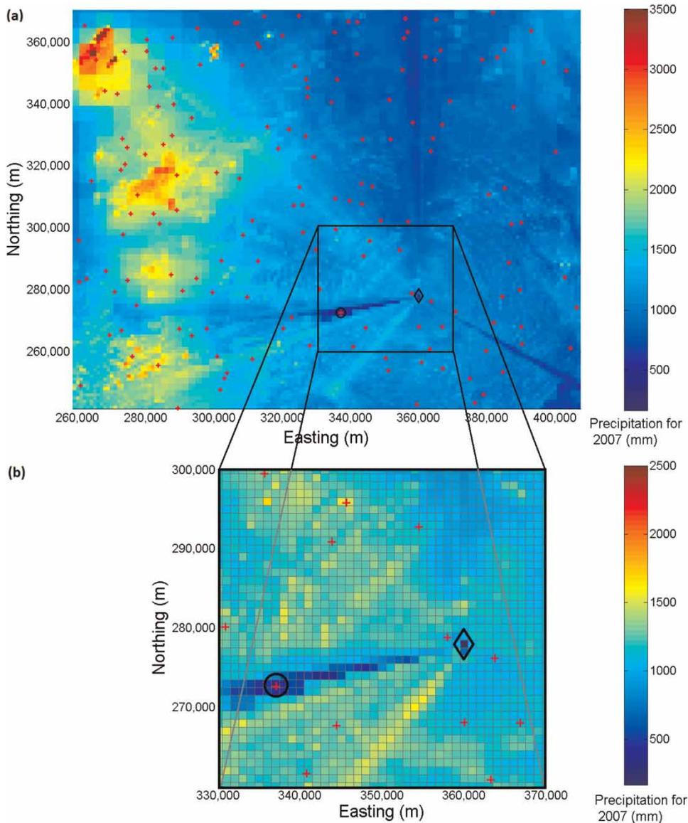
**Figure 4** | Accumulation of precipitation over the Upper Severn study area from NIMROD rainfall radar for 2007. The locations of the daily MIDAS rain gauges are marked (+). The rain gauge circled is located at MIDAS station 440885 (Brampton Bryan, 337100E, 272600N), this corresponds to the outlier circled in Figure 3. Clee Hill radar (◇ diamond) is located at 359485E, 277940N (Met Office 2009). Pixel size is 1 km<sup>2</sup>.
