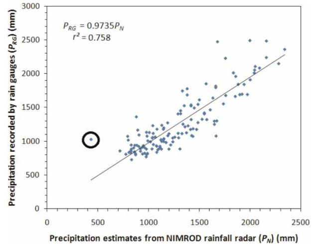
**Figure 3** | Comparison between NIMROD rainfall radar accumulations ( $P_N$ ) and MIDAS daily rain gauge readings ( $P_{RG}$ ) for 2007 for the Upper Severn Area, UK. Data from BADC (2010b). The outlier, circled, is the rain gauge at MIDAS station 440885 (Brampton Bryan, 337100E, 272600N).
