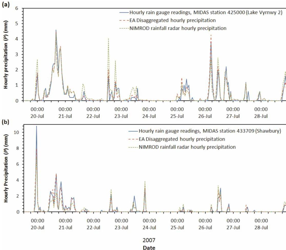
**Figure 7** | Time series of hourly precipitation ( $P$ ) from (a) MIDAS station 425000 (Lake Vyrnwy 2 E: 301,200 N: 318,700), EA disaggregated data from grid square centred on E: 301,000 N: 319,000, NIMROD radar data from grid square centred on 301500E, 318500N and (b) MIDAS station 433709 (Shawbury 355300E, 322100N), EA disaggregated data from grid square centred on 355000E, 322000N, NIMROD radar data from grid square centred on 355500E, 322500N. Rain gauge data from MIDAS (2010).
