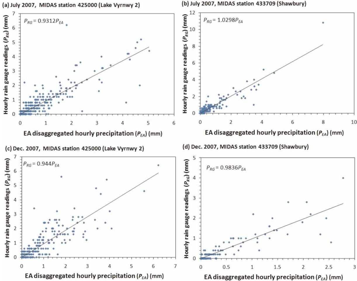
**Figure 6** | Comparison between EA disaggregated hourly precipitation ( $P_{EA}$ ) and MIDAS hourly rain gauge readings ( $P_{RG}$ ) for (a & b) July 2007 and (c & d) December 2007. (a & c) MIDAS station 425000 (Lake Vyrnwy 2, 301200E, 318700N), EA disaggregated data from grid square centred on 301000E, 319000N. (b & d) MIDAS station 433709 (Shawbury, 355300E, 322100N), EA disaggregated data from grid square centred on 355000E, 322000N. Rain gauge data from MIDAS (2010).
