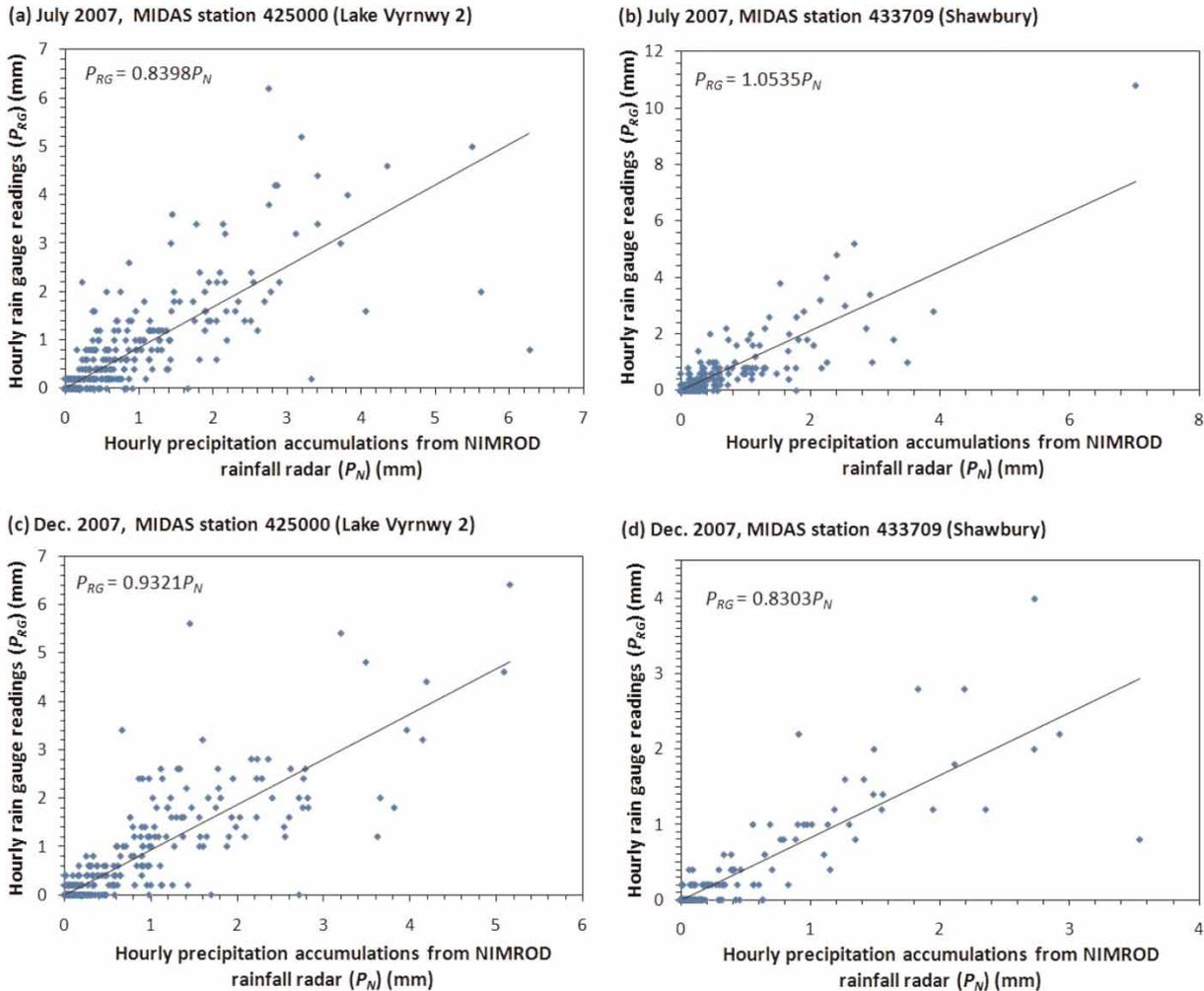
**Figure 5** | Comparison between NIMROD rainfall radar hourly accumulations ( $P_N$ ) and MIDAS hourly rain gauge readings ( $P_{RG}$ ) covering the periods (a & b) July 2007 and (c & d) December 2007. (a & c) MIDAS station 425000 (Lake Vyrnwy 2, 301200E, 318700N), NIMROD radar data from grid square centred on 301500E, 318500N. (b & d) MIDAS station 433709 (Shawbury, 355300E, 322100N), NIMROD radar data from grid square centred on 355500E, 322500N. Rain gauge data from MIDAS (2010).
