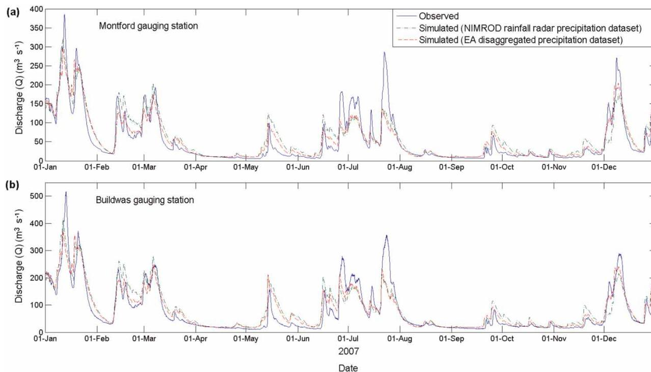
**Figure 8** | Observed and simulated discharge ( $Q$ ) for 2007 at (a) Montford and (b) Buildwas gauging stations on the upper reaches of the River Severn, UK. The simulation was performed using the LISFLOOD-RR hydrological model with the NIMROD rainfall radar and EA disaggregated hourly precipitation maps.
