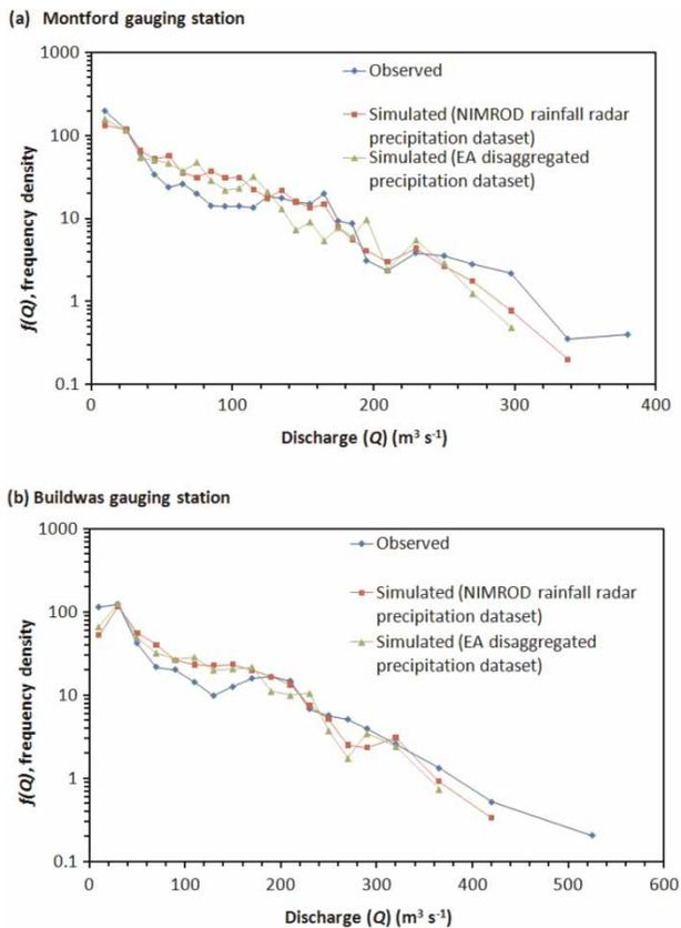
**Figure 9** | Frequency densities (number of occurrences of hourly discharge within a given range (bin) divided by the bin size) of the observed and simulated discharges ( $Q$ ) for 2007 at (a) Montford and (b) Buildwas gauging stations on the upper reaches of the River Severn.
