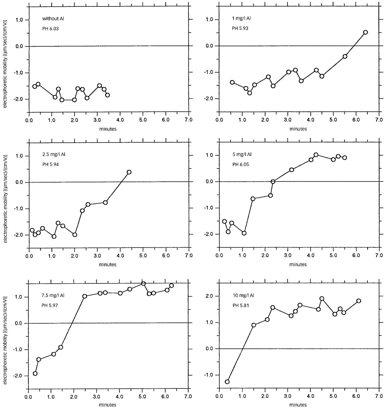
Figure 11 | EM of *Synechocystis* cells at pH 6 during a period of 7 min and increasing alum dosage (0, 1, 2.5, 5, 7.5 and 10 mg/l).
