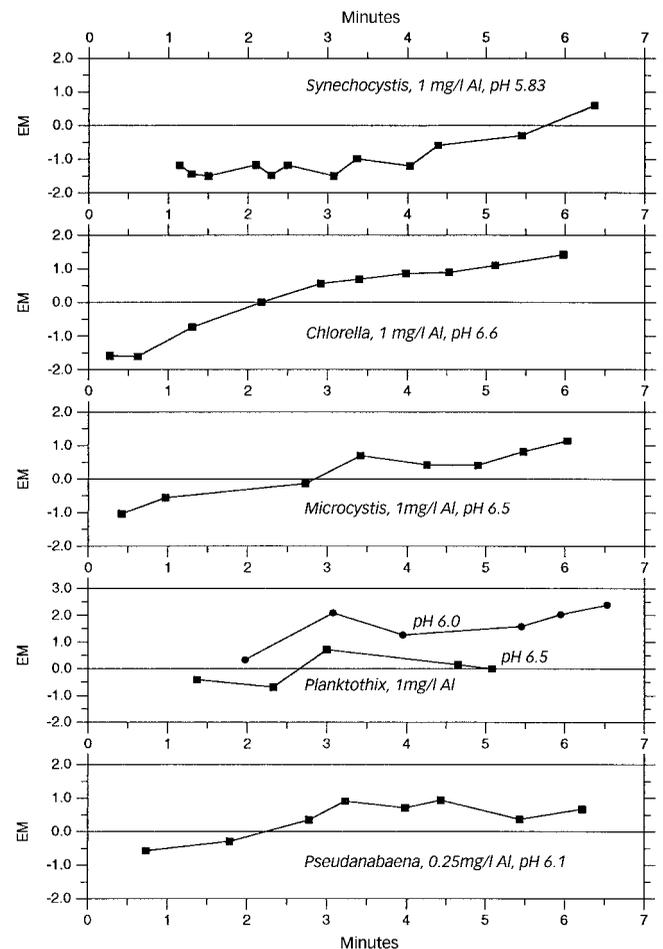
**Figure 5** | EM of different algal species after addition of flocculant during a period of 7 min. From more than 20 experiments per species these curves were chosen, which demonstrate a charge reversal with the lowest concentration of alum.
