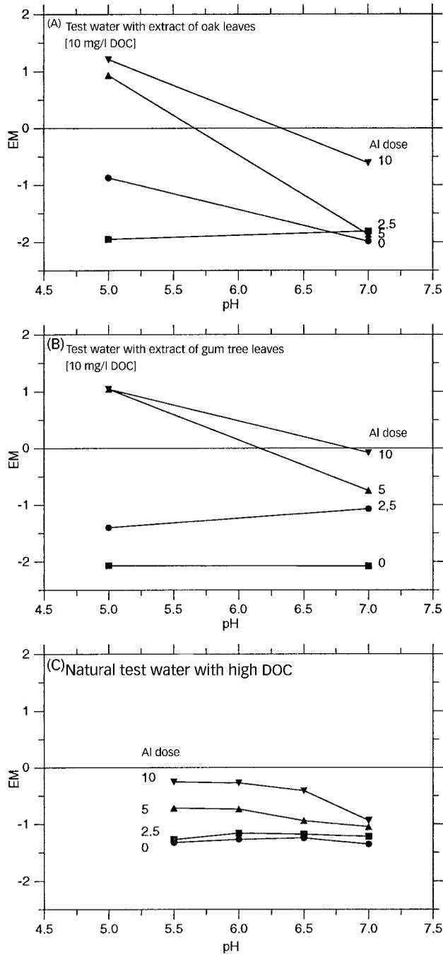
**Figure 10** | EM of *Synechocystis* cells in waters with high concentrations of DOC with increasing pH and alum dosage (0, 2.5, 5, 10 mg/l).
