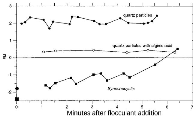
**Figure 4** | EM of quartz particles with and without alginic acid in comparison with *Synechocystis* cells during a period of 7 min. All experiments were run at pH 6 with 1 mg/l alum dosage. Boxes at time zero give the initial charge of algae and quartz particles.
