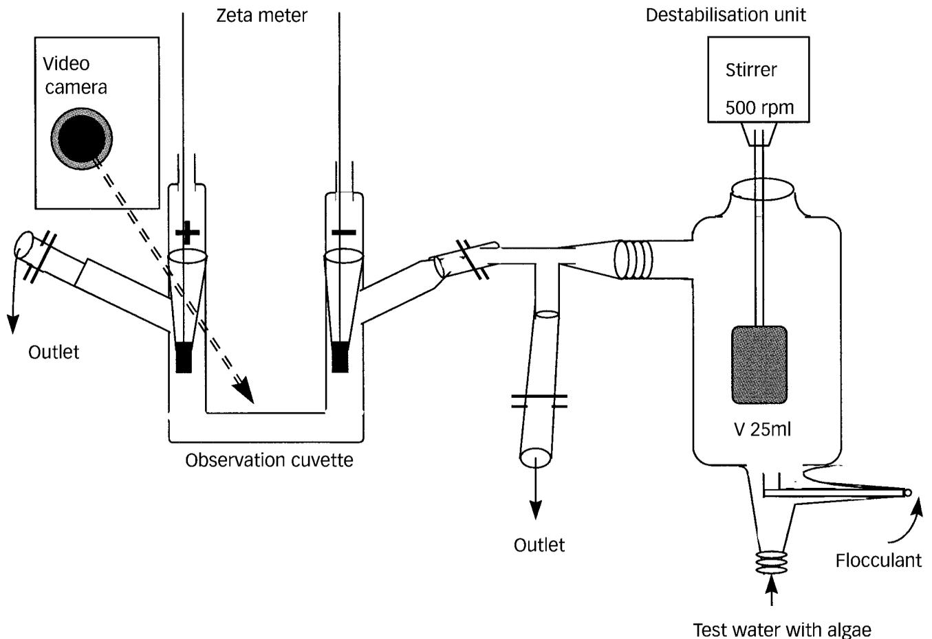
**Figure 1** | A schematic diagram of the destabilisation unit and the modified observation cuvette of the Zeta meter.
