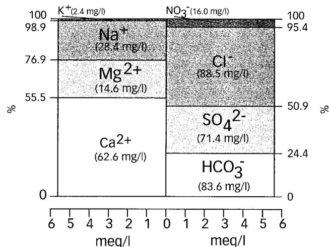
**Figure 2** | Composition of ions in test water used for experiments.
