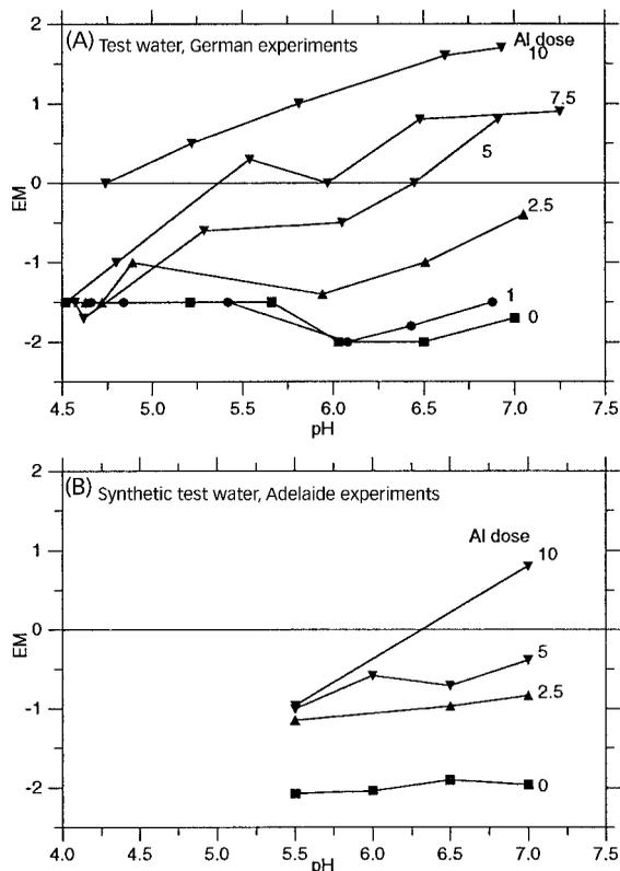
**Figure 7** | EM of *Synechocystis* cells is shown with increasing pH values (4.5, 5, 5.5, 6, 6.5, 7) and alum concentrations (1, 2.5, 5, 7.5, 10 mg/l) in test water. (A) German experiments: EM is given as 2 min values interpolated from time-dependent curves; (B) Australian experiments: EM is given as 2 min averages ( $n > 17$  measurements).
