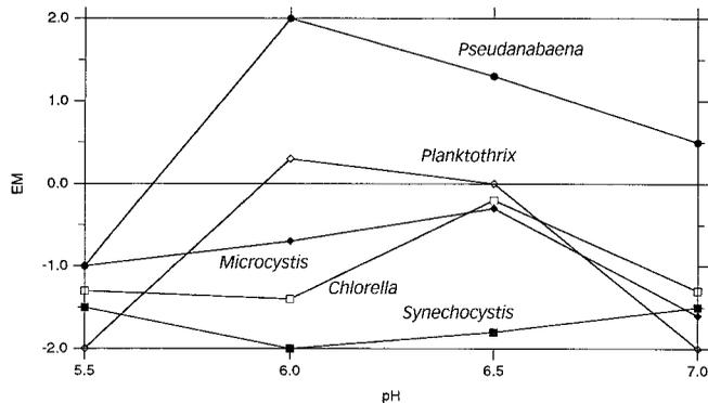
**Figure 9** | 2 min values of EM for five algal species with increasing pH and an alum dosage of 1 mg/l in test water (pH values are optimised).
