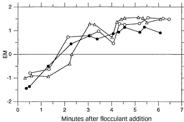
**Figure 3** | EM of *Synechocystis* cells at different times after destabilisation in three replicates. Conditions of experiments were similar with 5 mg/l alum and pH values between 6.45 and 6.55.
