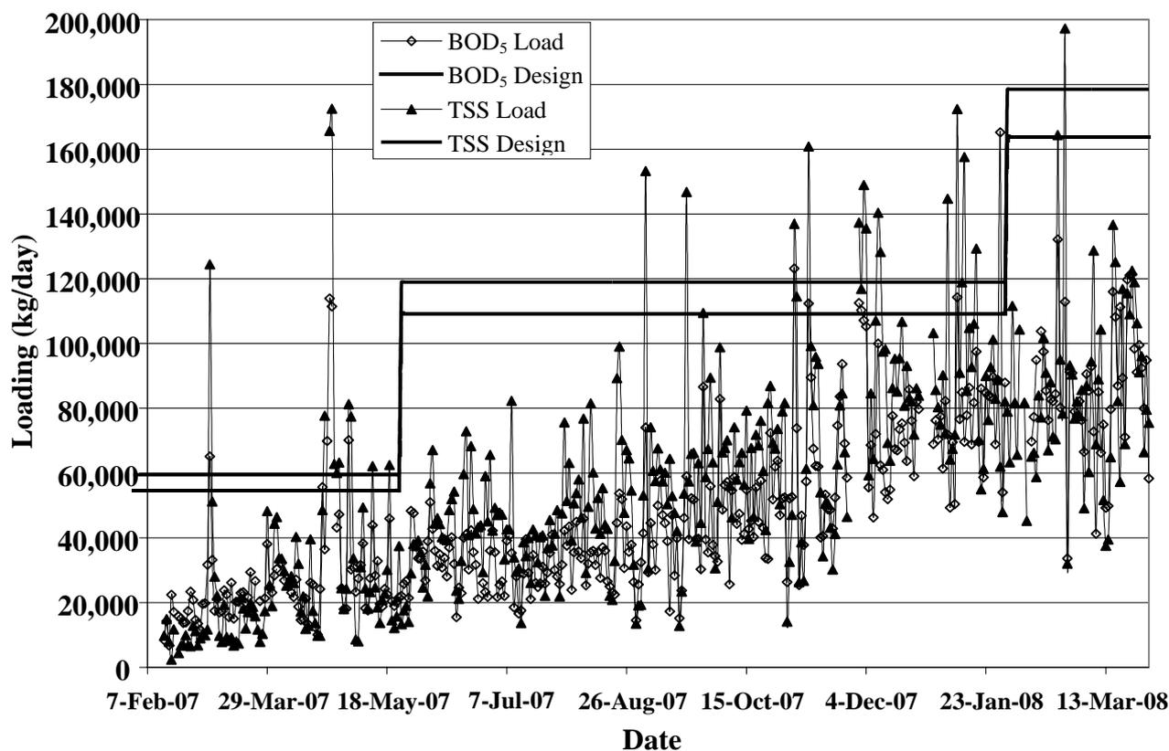
Figure 4. CWRP Influent Waste Loadings in Comparison to Design Values.
