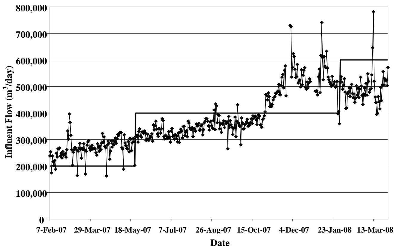
**Figure 3.** CWRP Influent Flow in Comparison to Nominal Design Values.
