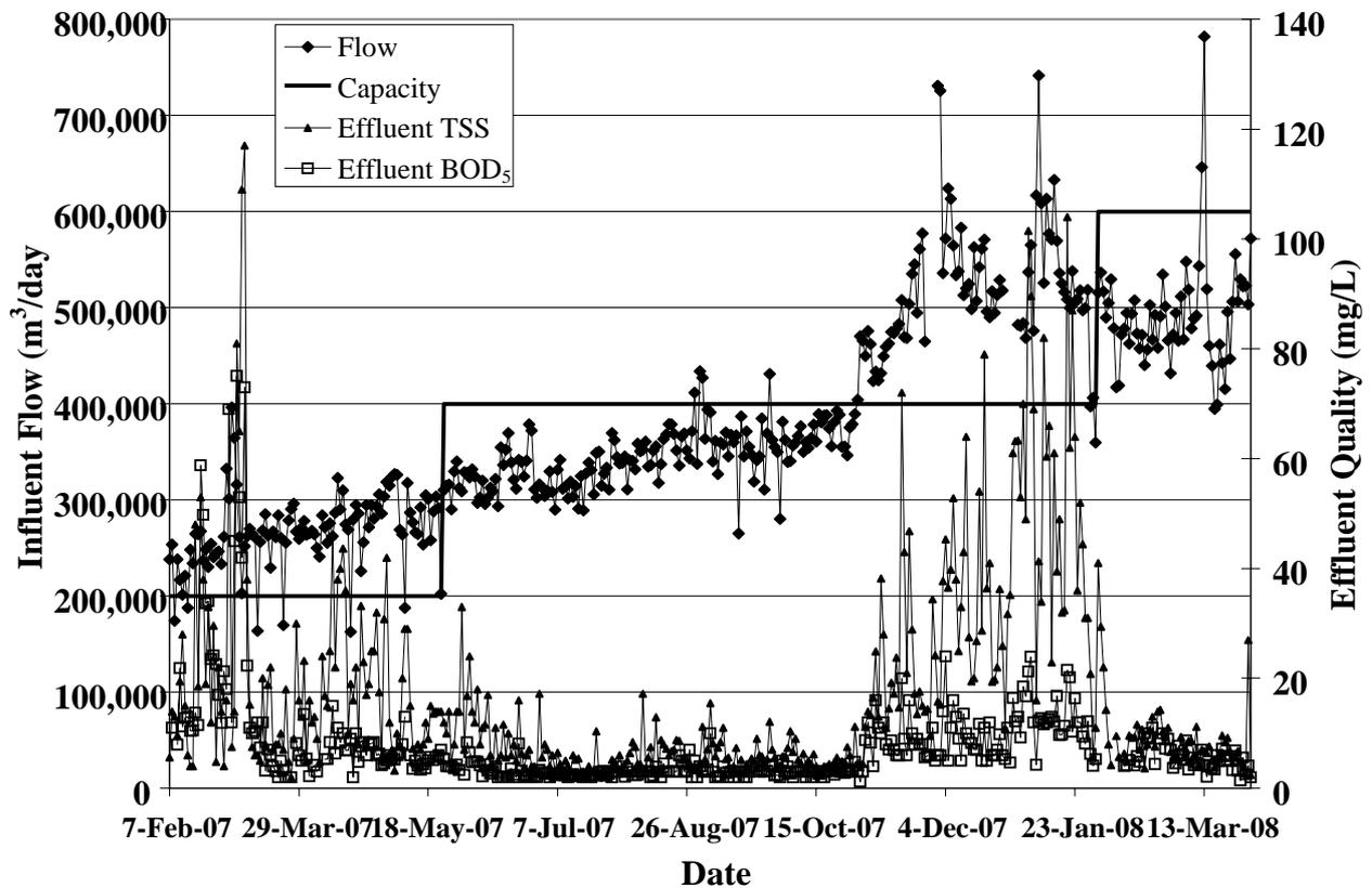
**Figure 5.** CWRP Effluent BOD<sub>5</sub> and TSS, with Plant Flow and Capacity Shown for Comparison.
