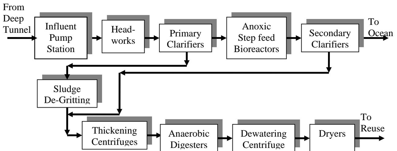
**Figure 1.** CWRP Process Flow Diagram.
