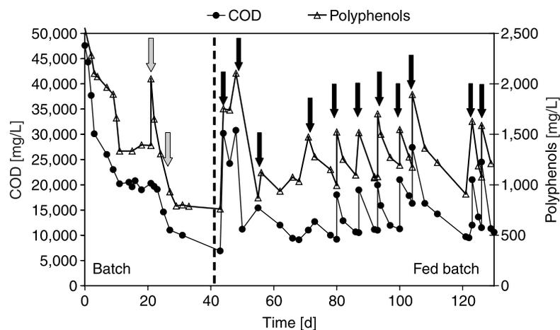
**Figure 2** COD and TP concentration trends in the aerobic batch reactor. The grey arrows indicate pure phenolic compounds injections in the reactor, the black arrows indicate OMW injections
