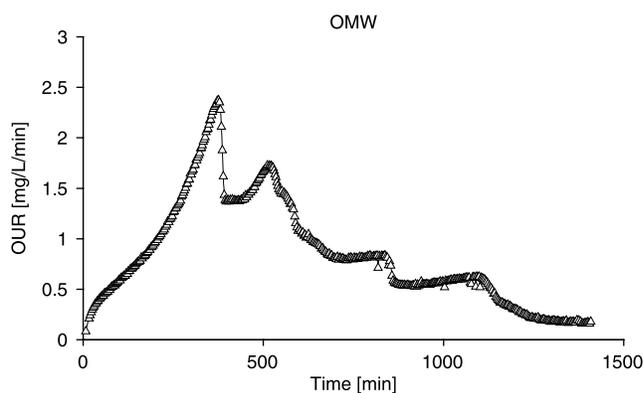
**Figure 3** Respirometric test obtained adding 100 mL of OMW to the fungi biomass
