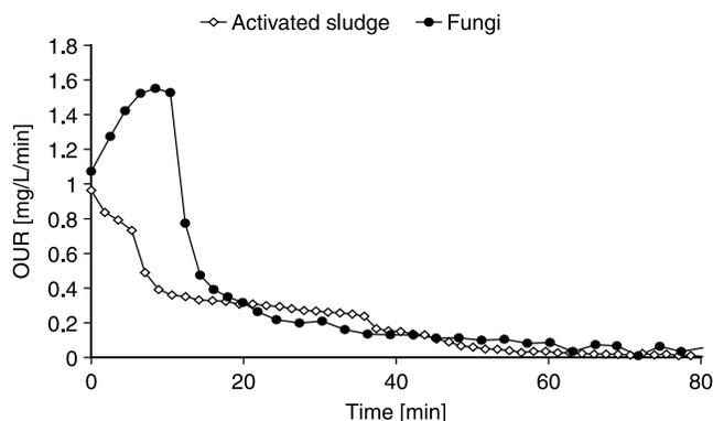
**Figure 4** OMW respirometric tests with fungi and activated sludge biomass
