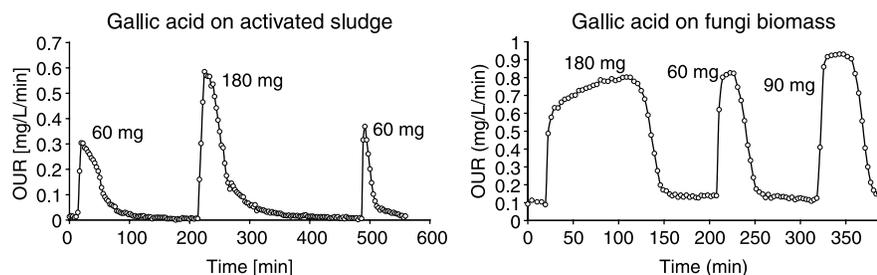
**Figure 6** Repeated injections of gallic acid on activated sludge (left) and on fungi biomass (right)
