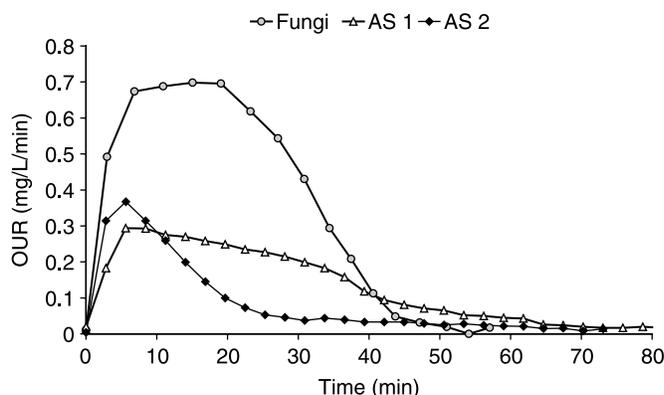
**Figure 7** Respirograms obtained with 60 mg gallic acid injections on activated sludge and fungi biomass
