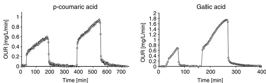
**Figure 5** Respirometric tests obtained adding p-coumaric acid (left) and gallic acid (right) to the fungi biomass**Table 7** Kinetic and stoichiometric parameters of fungi biomass
