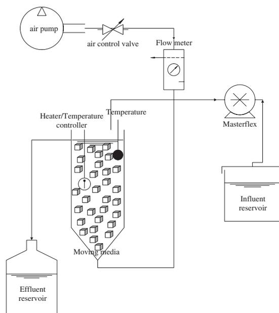
**Figure 1** Schematic diagram of laboratory reactor system
