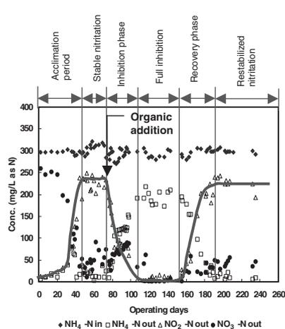
**Figure 3** Nitrogen profiles in nitrification reactor 2 with COD 156 mg/L and  $\text{NH}_4^+\text{-N}$  297 mg/L
