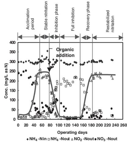
**Figure 4** Nitrogen profiles in nitrification reactor 3 with COD 299 mg/L and  $\text{NH}_4^+\text{-N}$  298 mg/L
