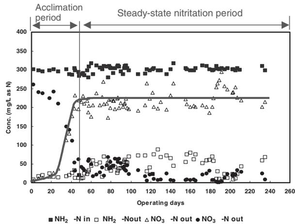
**Figure 2** Nitrogen profiles in nitrification reactor 1 with COD 0 mg/L and  $\text{NH}_4^+\text{-N}$  301 mg/L
