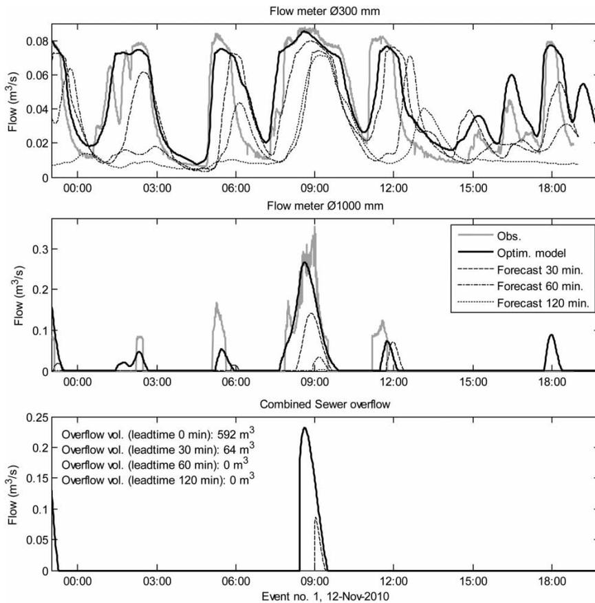
**Figure 5** | Example of observed, modeled (optimized), and forecasted flows with different lead times corresponding to the location of the small flow meter (top panel), the large flow meter (middle panel), and the combined sewer overflow (bottom panel). Event 1: 12 Nov 2010.
