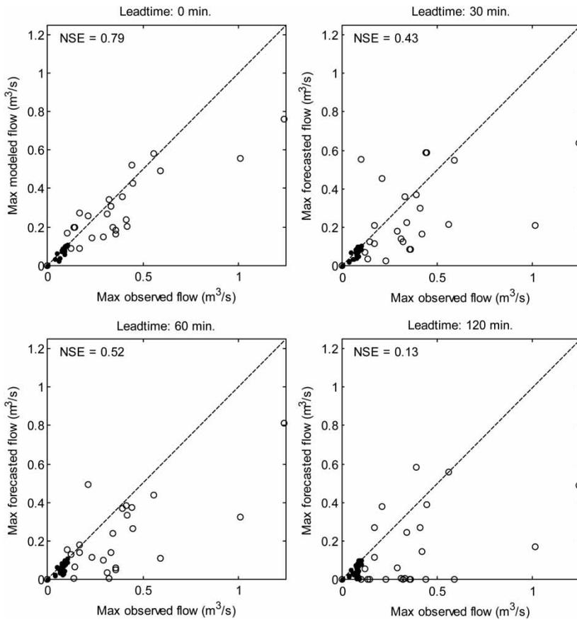
**Figure 4** | Top left panel: Observed vs. modeled (optimized) peak flows. Other panels: Observed vs. forecasted peak flows with different lead times. Solid dots mark the flow in the small ( $\varnothing 300$  mm flow meter) and the hollow dots mark the large ( $\varnothing 1,000$  mm) flow meter.
