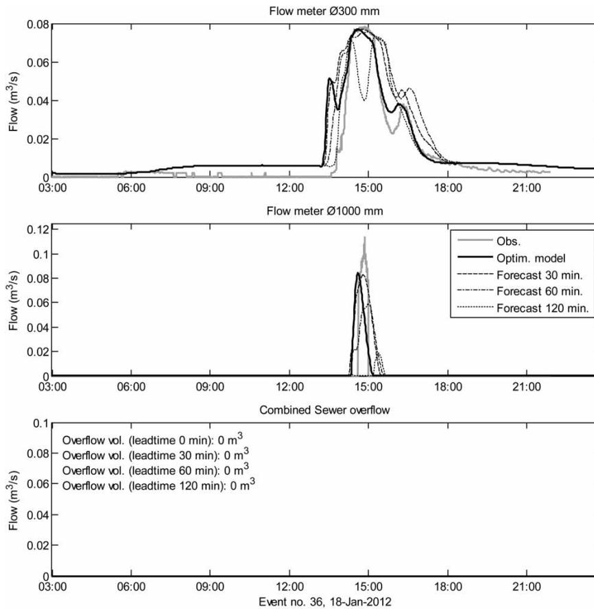
**Figure 6** | Example of observed, modeled (optimized), and forecasted flows with different lead times corresponding to the location of the small flow meter (top panel), the large flow meter (middle panel), and the combined sewer overflow (bottom panel). Event 36: 18 Jan. 2012.
