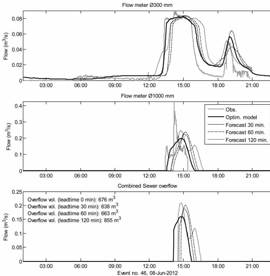
**Figure 7** | Example of observed, modeled (optimized), and forecasted flows with different lead times corresponding to the location of the small flow meter (top panel), the large flow meter (middle panel), and the combined sewer overflow (bottom panel) Event 46: 8 June 2010.
