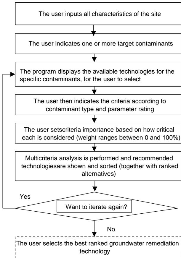
Figure 4 | General algorithm supported with CCR.
