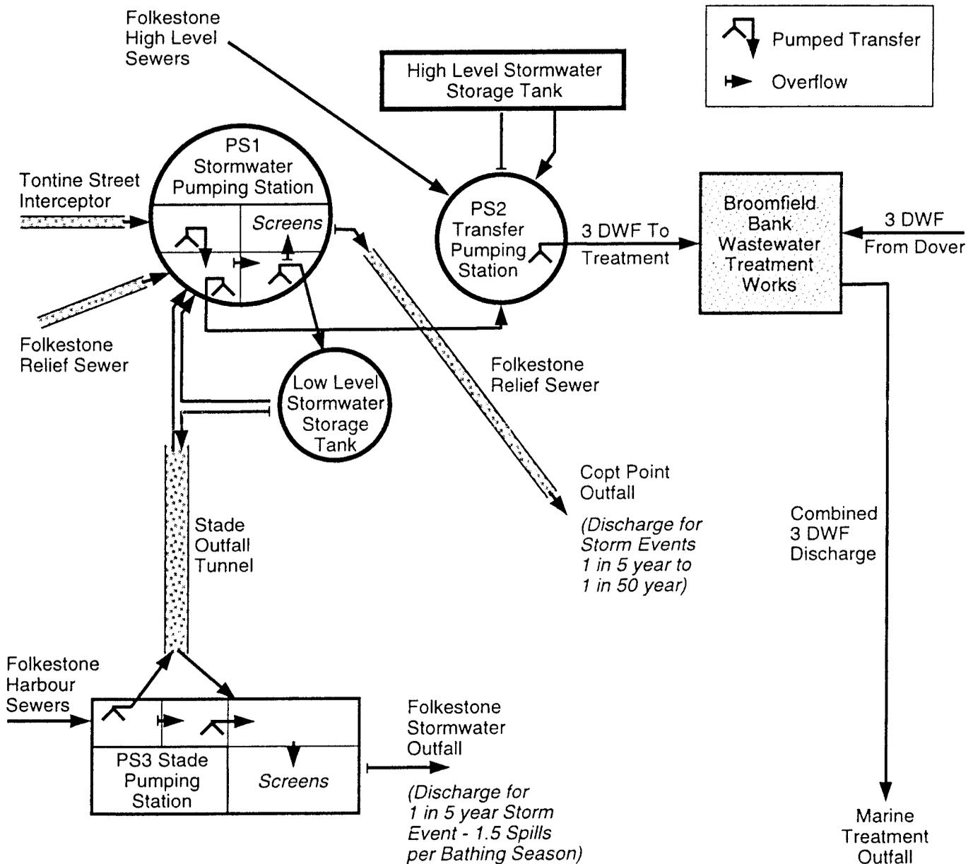
Figure 2 | Folkestone Junction flow schematic.
