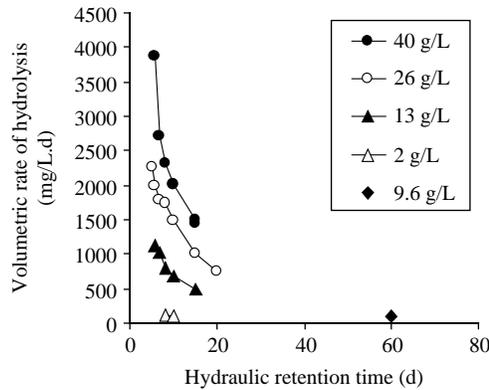
**Figure 2** Plot of the calculated rate of hydrolysis for each steady state as a function of the hydraulic retention time, showing the effect of the feed COD concentration
