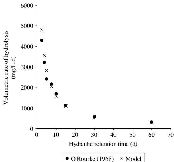
**Figure 4** Calculated (from experimental data) and predicted (first order kinetics,  $k_h = 0.992d^{-1}$ ) rate of hydrolysis for each hydraulic retention time for the data of O'Rourke (1968)
