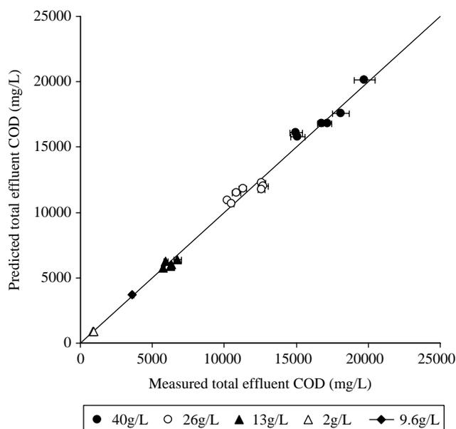
**Figure 3** Plot of the calculated effluent COD concentration assuming first order kinetics with  $k_h = 0.992\text{d}^{-1}$  versus the measured effluent COD concentration
