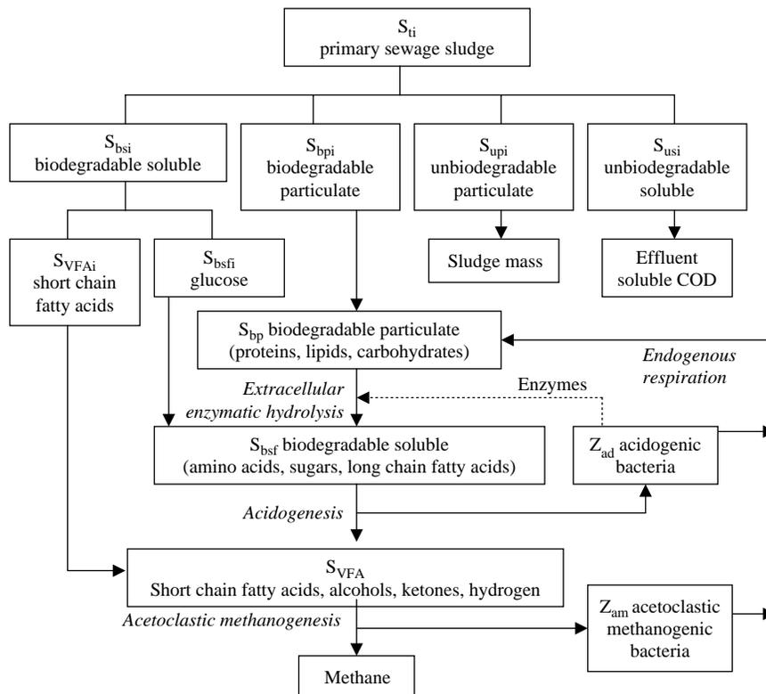
**Figure 1** Schematic diagram (in units of COD) of the bulk processes involved in the anaerobic digestion of primary sewage sludge
