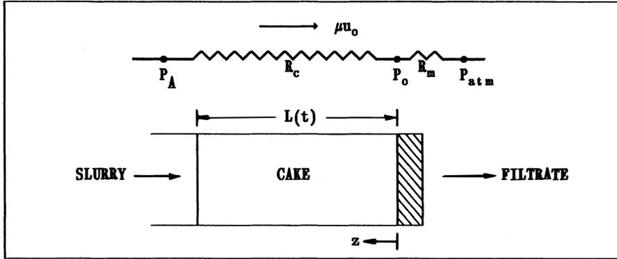
Fig. 1. Electrical resistance analogy of filtration.
