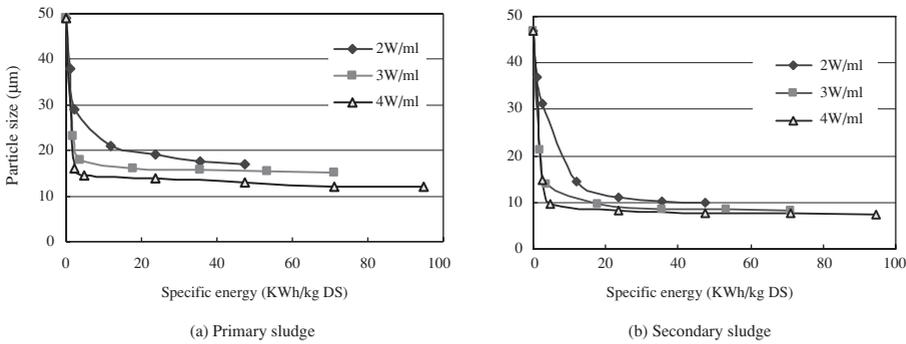
**Figure 6** Effects of specific energy on particle size at different ultrasound densities
