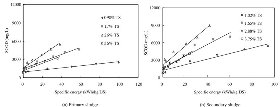
**Figure 9** Specific energy vs SCOD increase at different solids concentrations
