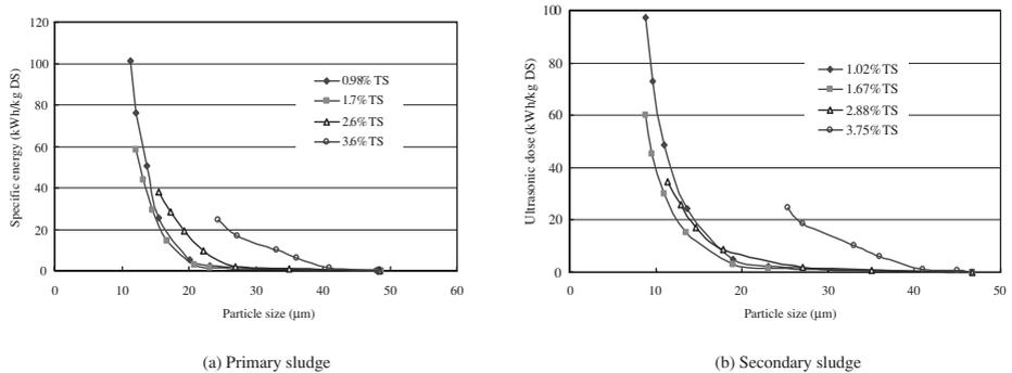
**Figure 8** Specific energy vs particle size reduction at different solids concentrations
