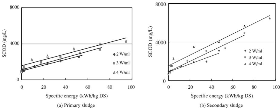
**Figure 7** Effects of specific energy on SCOD at different ultrasound densities
