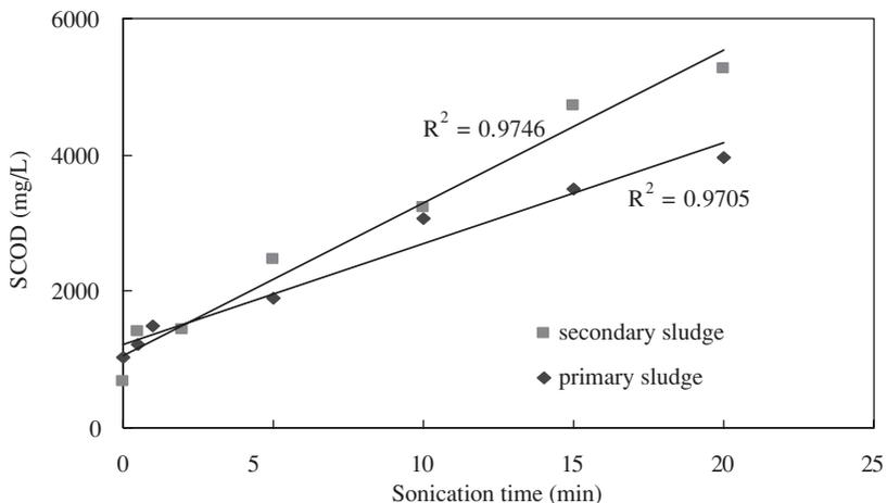
**Figure 4** SCOD increase of primary and secondary sludge (3 W/ml)
