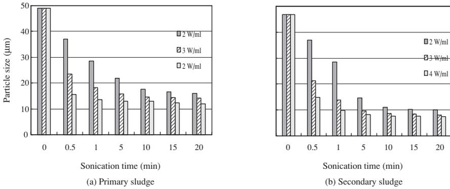
**Figure 5** Effects of particle size reduction at different ultrasound densities
