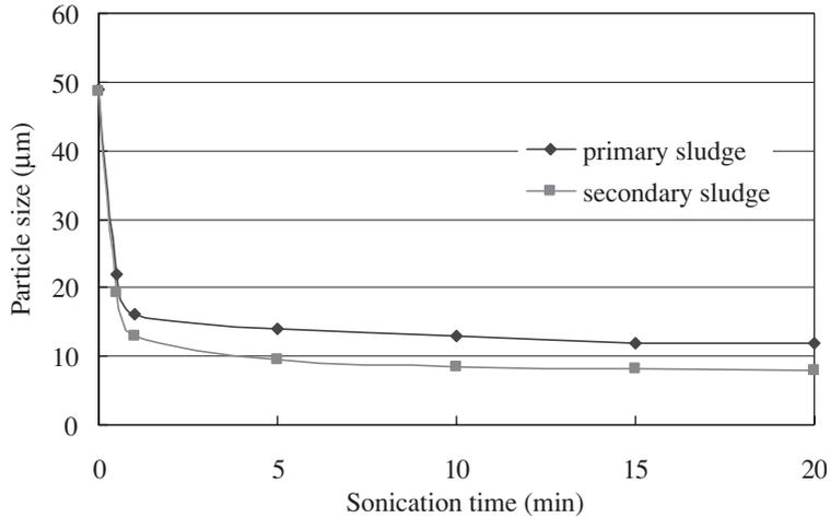
**Figure 3** The particle size reduction of primary and secondary sludge (3 W/ml)
