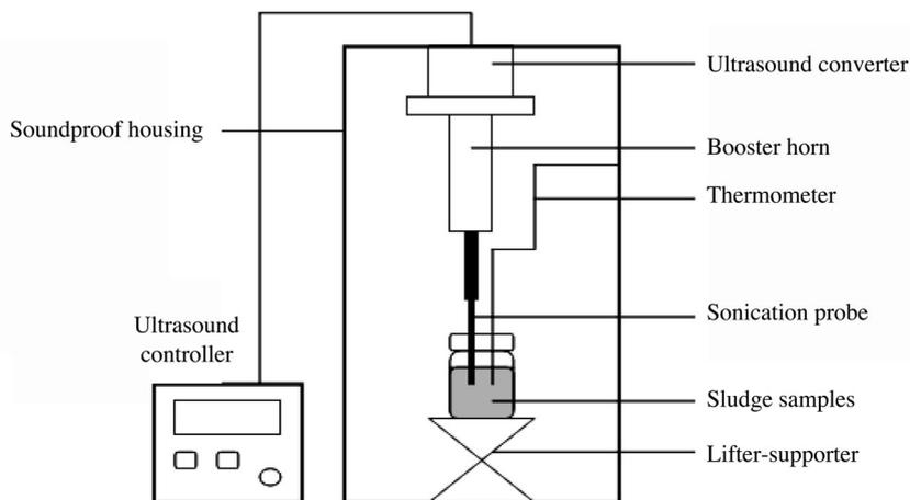
**Figure 1** Schematic diagram of ultrasound pretreatment
