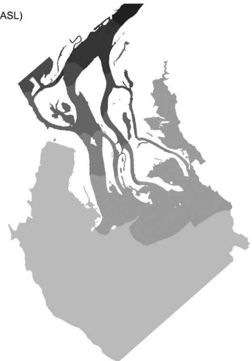
Figure 8 | Computed water levels for the flow situation of July 1997; free surface computation.
