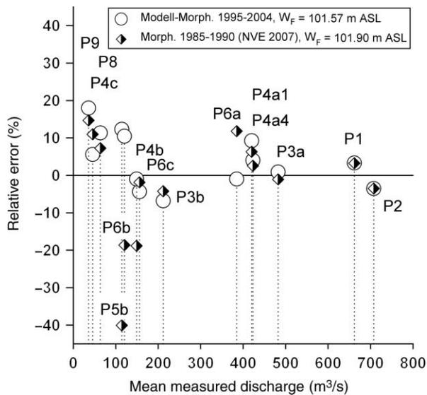
**Figure 9** | Relative errors of the computed discharges for different morphology datasets, flow situation from October 1996; for free surface and a maximum of 10 cells in vertical direction,  $W_F$  = water level at Fetsund Bru.
