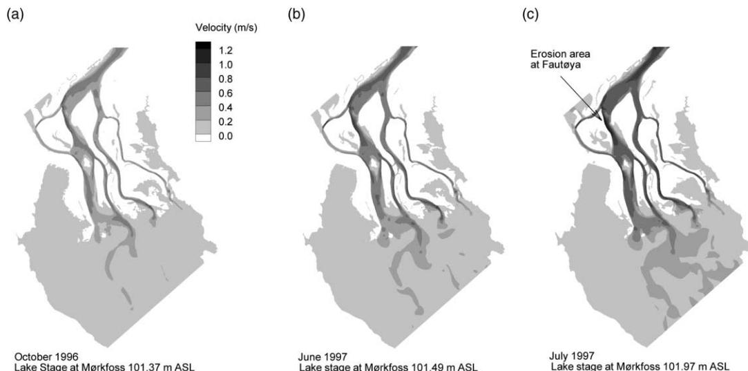
**Figure 10** | Computed flow velocities on the water surface for the flow situation of (a) October 1996, discharge  $712 \text{ m}^3/\text{s}$ , (b) June 1997, discharge  $1,036 \text{ m}^3/\text{s}$  and (c) July 1997, discharge  $1,496 \text{ m}^3/\text{s}$ ; free surface computations.
