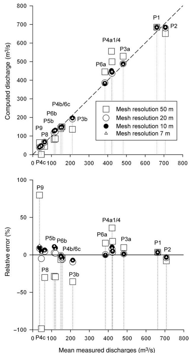
**Figure 6** | Computed versus measured discharges and relative errors for the flow situation from October 1996 for different spatial grid resolutions (fixed water surface at 101.47 m a.s.l.,  $k_s = 0.5$  m, maximum of 10 vertical cells).
