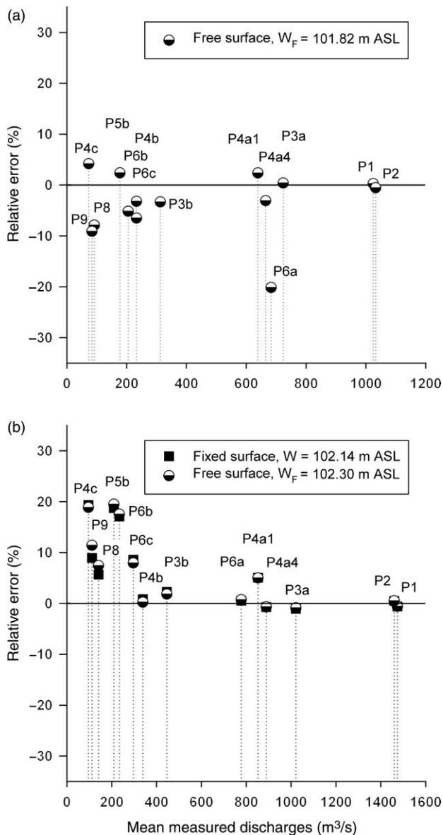
**Figure 7** | Relative errors of the computed discharges for the flow situation from (a) June 1997 and (b) July 1997;  $k_s = 0.2$  m, a maximum of 20 cells in vertical direction;  $W_F$  = water level at Fetsund Bru.
