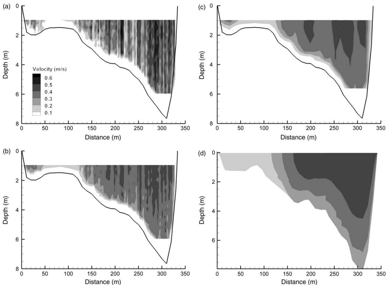
**Figure 11** | Flow velocities at profile P6a for the flow situation of October 1996: (a) average of two ADCP measurements, (b) average of eight ADCP measurements, (c) spatial aggregation of the average of eight ADCP measurements using a raster of 31 horizontal and 12 vertical cells and (d) mean flow velocities, computed with SSIIM for the model morphology from 1995–2004 (free surface computation).
