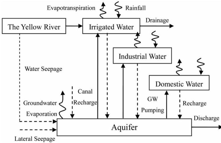
Figure 4 | Schematic diagram of the conjunctive use system.
