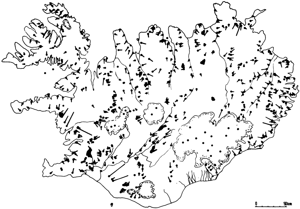
Fig. 1. Distribution of sampling points of precipitation, local groundwater and streams, and winter precipitation on glaciers in Iceland. The winter precipitation is collected before the beginning of the melting season. When only a black point is given the water is believed to originate as precipitation around the sampling point. In other cases a line has been drawn from the sampling point into the middle of the proposed recharge area.
