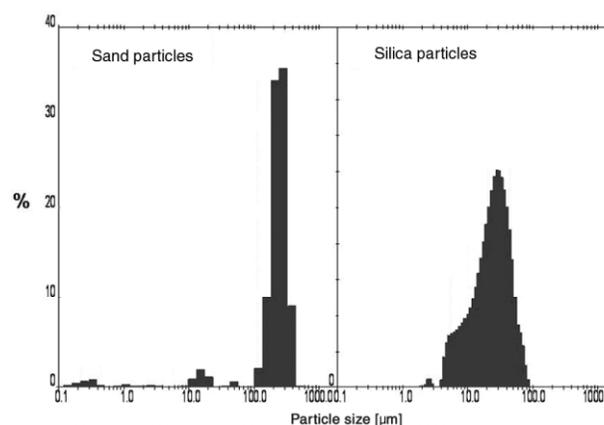
Figure 1 | Particle size distribution of the employed substrate materials.
