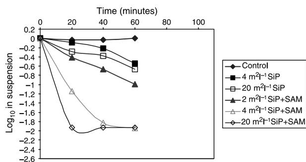
Figure 4 | Log<sub>10</sub> removal of MS-2 bacteriophage with silica powder and silica powder coated with SAM.
