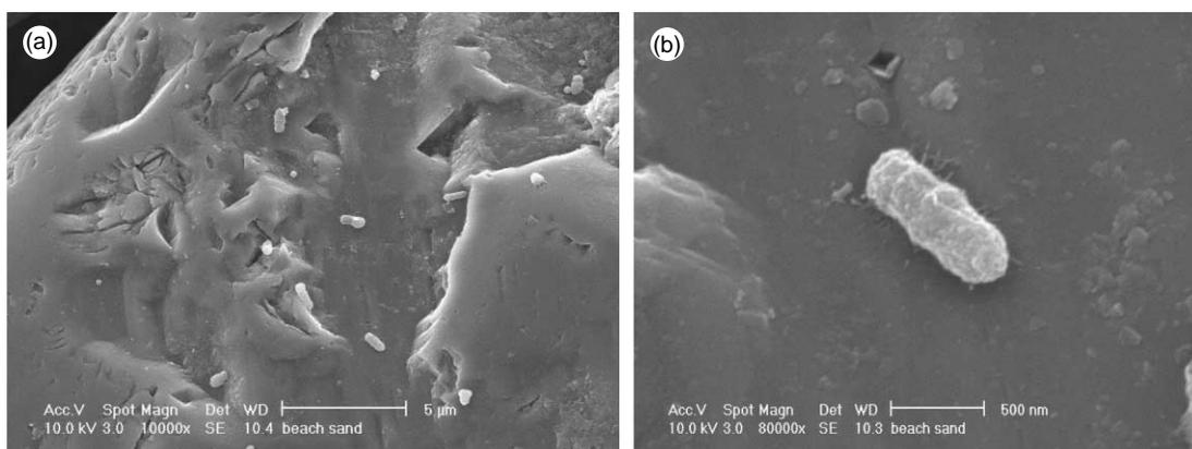
**Figure 6** | (a) and (b) SEM images of *E. coli* on SAM coated sand particles.
