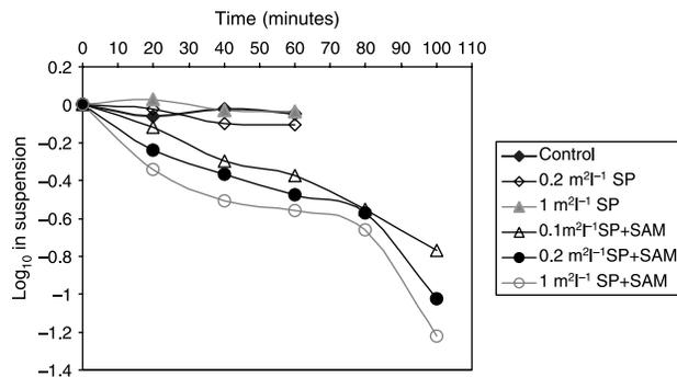
Figure 5 | Log<sub>10</sub> removal of MS-2 bacteriophage with sand particles and sand particles coated with SAM.
