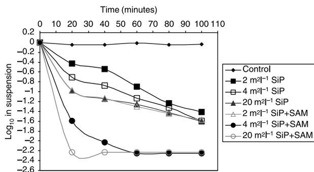
**Figure 2** |  $\log_{10}$  removal of *E. coli* with silica powder and silica powder coated with SAM.
