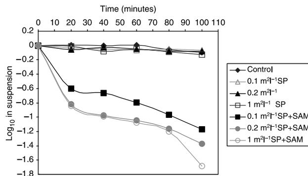
**Figure 3** |  $\log_{10}$  removal of *E. coli* with sand particles and sand particles coated with SAM.
