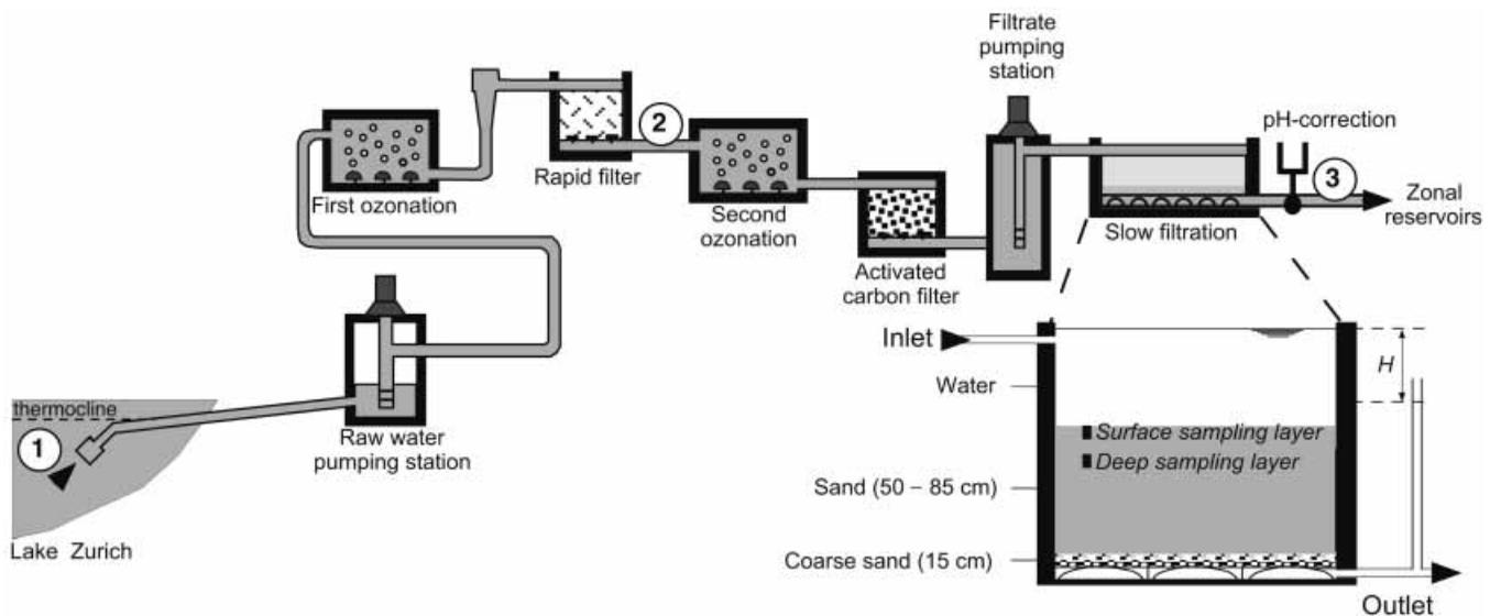
**Figure 1** | Water plant of Zurich-Lengg with a detailed profile of the slow sand filters. Sampling layers are indicated in italics.  $H$  is the total head loss throughout the filter.
