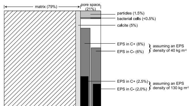
**Figure 7** | Schematic composition of a unit volume of the top layer of the sand filters, showing the volume fractions attributed to the individual clogging processes. EPS values are averages of the three sampling dates.
