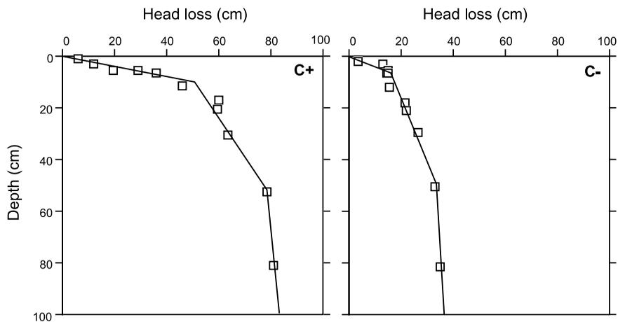
**Figure 4** | Depth profile of the head loss for filters SSF2 and SSF10 as representatives of C+ and C- filters, respectively, based on measurement of piezometric levels in August 2001.
