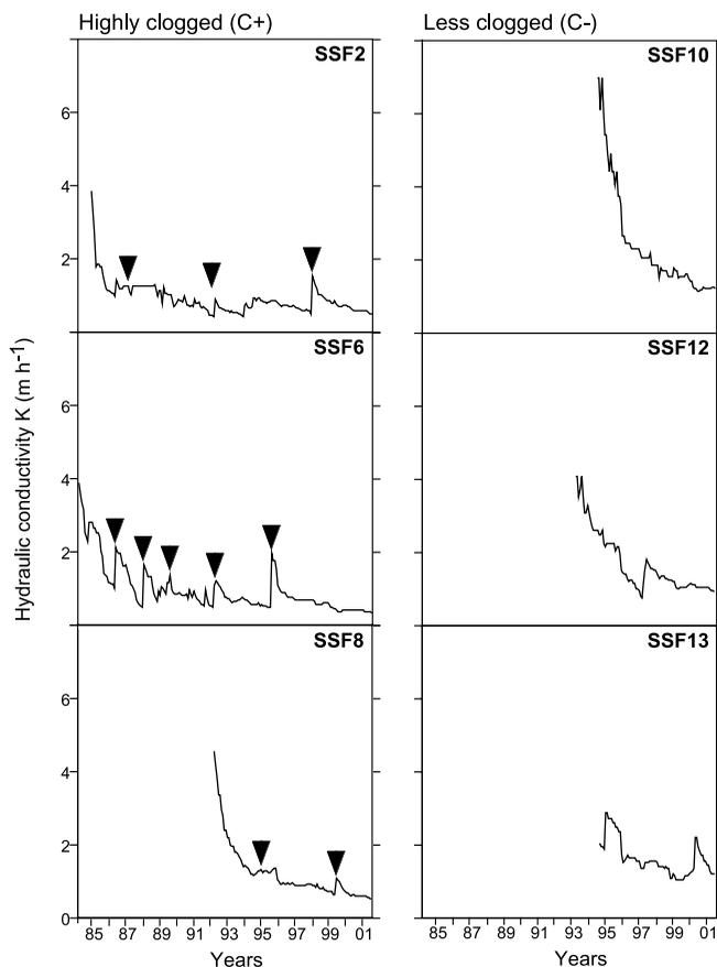
**Figure 2** | Evolution of hydraulic conductivity for highly and less clogged filters based on measured head differences from inlet to outlet with a constant water flow of  $500 \text{ m}^3 \text{ h}^{-1}$ . Arrows indicate cleaning by removing the top 5 cm of sand.
