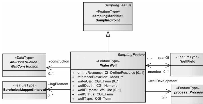
Figure 9 | GWML logical schema fragment for water wells.
