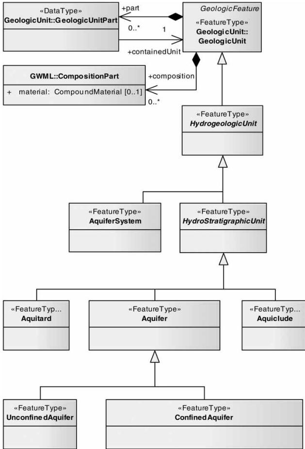
Figure 8 | GWML logical schema fragment for aquifers.
