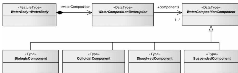
Figure 7 | GWML logical schema for water body and its composition.
