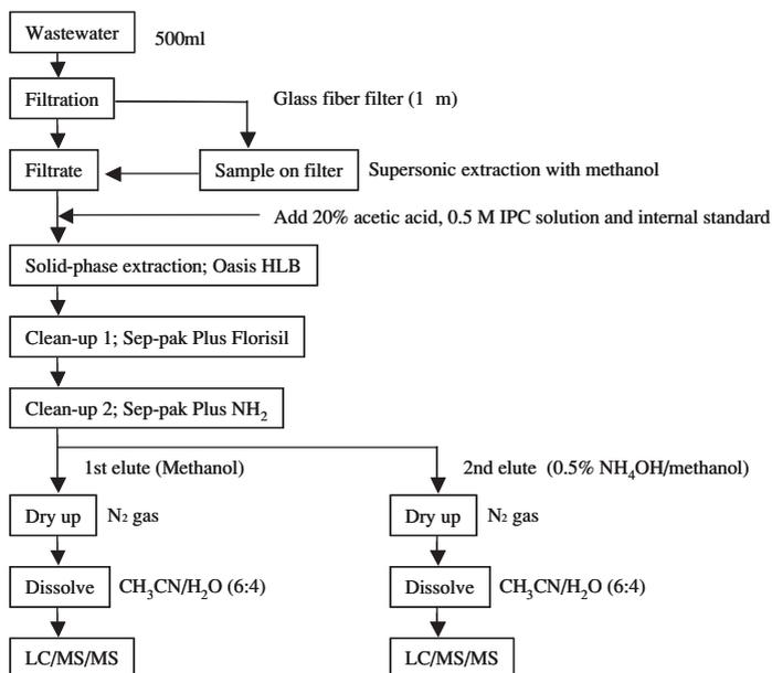
**Figure 1** Flow diagram of analytical method
