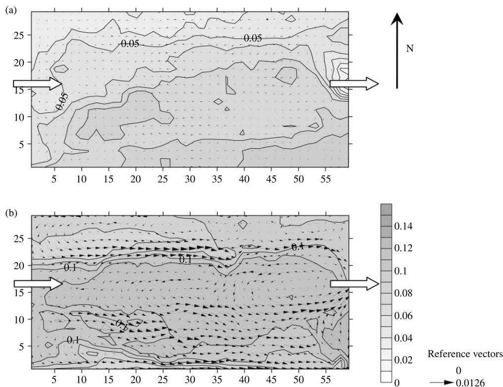
**Figure 3** | Layout 1. Water velocity ( $\text{m s}^{-1}$ ) and tracer concentration ( $\text{g m}^{-3}$ ) at the bottom (a) and the surface (b) of the pond 12 h after injection, the wind coming from the West at a  $2 \text{ m s}^{-1}$  speed.
