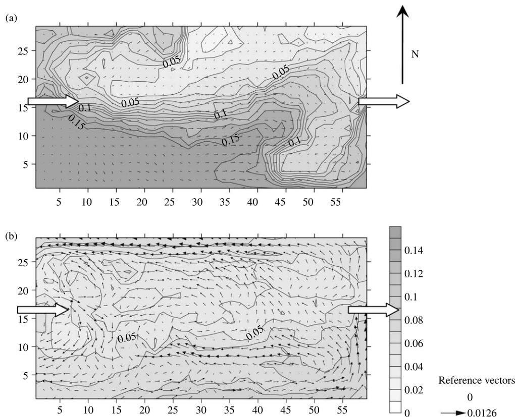
**Figure 4** | Layout 1. Water velocity ( $\text{m s}^{-1}$ ) and tracer concentration ( $\text{g m}^{-3}$ ) at the bottom (a) and the surface (b) of the pond 12 h after injection, the wind coming from the East at a  $2 \text{ m s}^{-1}$  speed.
