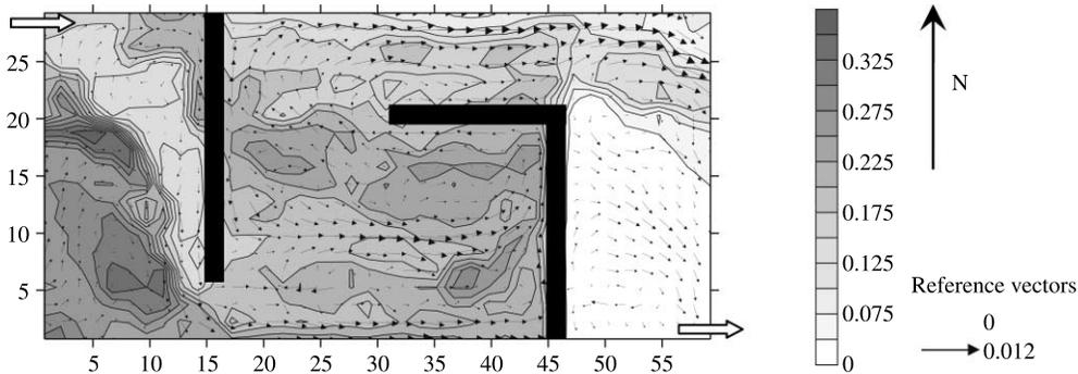
**Figure 7** | Layout 4. Water velocity ( $\text{m s}^{-1}$ ) and tracer concentration ( $\text{m}^{-3}$ ) at the pond surface, 12 h after injection, for a wind coming from the West, at a speed of  $2 \text{ m s}^{-1}$ .
