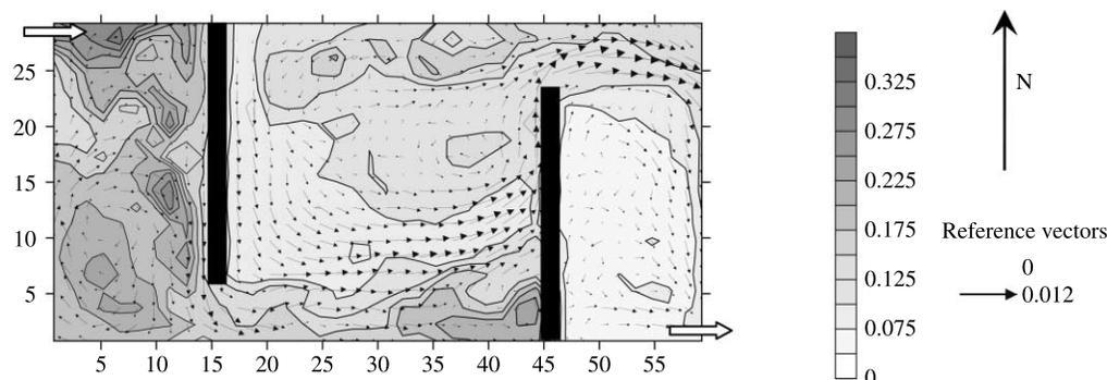
**Figure 6** | Layout 3. Water velocity ( $\text{m s}^{-1}$ ) and tracer concentration ( $\text{m}^{-3}$ ) at the pond surface, 12 h after injection, for a wind coming from the West, at a speed of  $2 \text{ m s}^{-1}$ .
