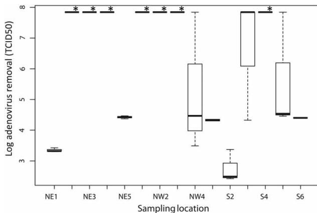
**Figure 4** | Removal of adenovirus spiked in drinking water samples (10 L) processed by the multi-barrier device. The boxes show the variability between replicates and dashed lines the data distribution. \*Adenovirus removal for these samples was below the method limit of detection.
