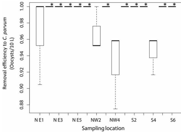
**Figure 6** | Removal of *Cryptosporidium parvum* oocysts spiked in drinking water samples (10 L) processed by the multi-barrier device. The boxes show the variability between replicates and dashed lines the data distribution. \*Oocyst removal for these samples was below the method limit of detection.
