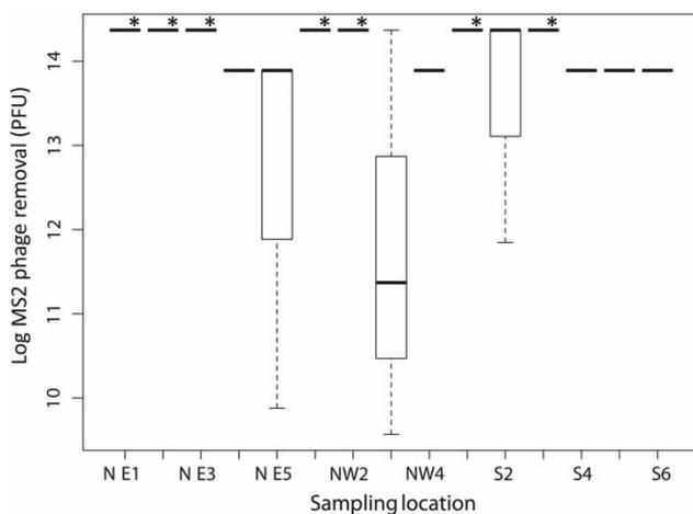
**Figure 3** | Removal of MS2 spiked in drinking water samples (10 L) processed by the multi-barrier device. The boxes show the variability between replicates and dashed lines the data distribution. \*MS2 removal for these samples was below the method limit of detection.
