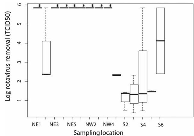
**Figure 5** | Removal of rotavirus spiked in drinking water samples (10 L) processed by the multi-barrier device. The boxes show the variability between replicates and dashed lines the data distribution. \*Rotavirus removal for these samples was below the method limit of detection.
