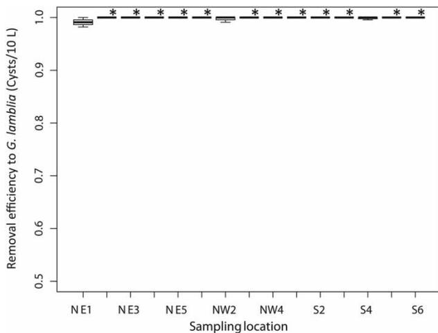
**Figure 7** | Removal of *Giardia lamblia* cysts spiked in drinking water samples (10 L) processed by the multi-barrier device. The boxes show the variability between replicates and dash lines the data distribution. \*Cyst removal for these samples was below the method limit of detection.
