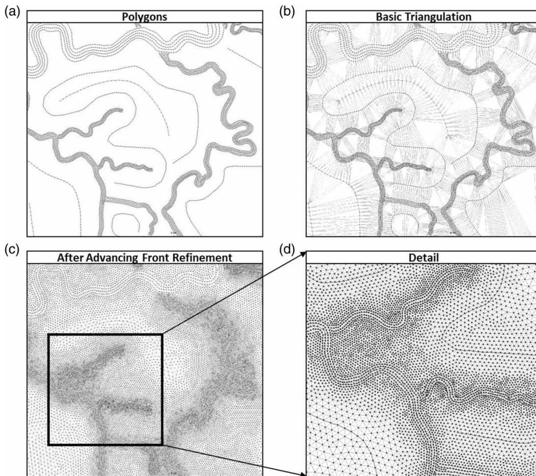
Figure 8 | Mesh triangulation steps: (a) defining the desired node distance for specific areas on forcing polygons; (b) initial triangulation; (c) and (d) advancing front step that iteratively refined the mesh while protecting nodes on the forcing polygons.
