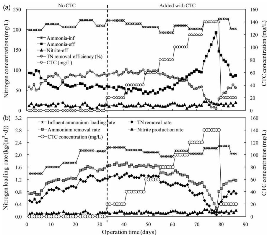
**Figure 5** | (a) Concentrations of nitrogen compounds during the single-stage ANAMMOX process under different CTC concentrations. (b) Removal and production rates of nitrogen compounds during the single-stage ANAMMOX process under different CTC concentrations.
