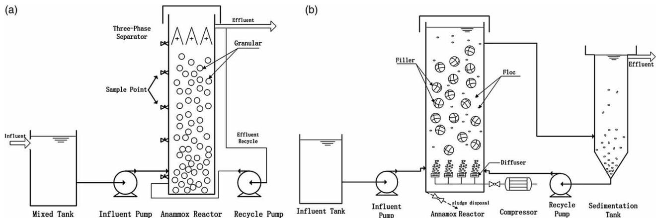
Figure 1 | Flow chart of (a) conventional ANAMMOX and (b) single-stage ANAMMOX.
