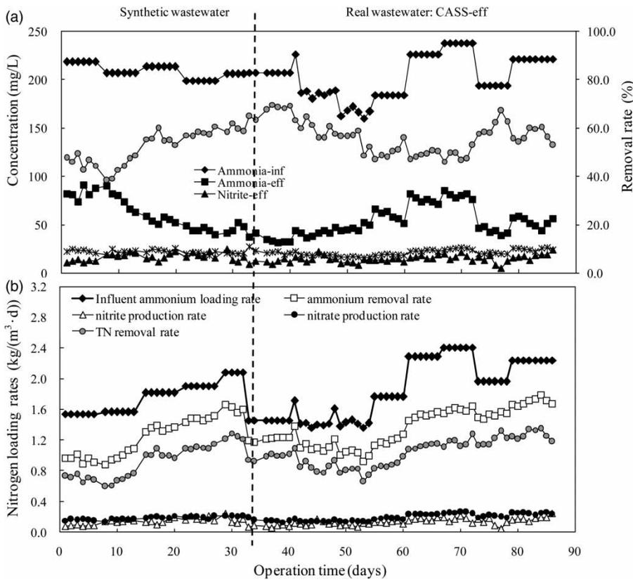
**Figure 4** | (a) Concentrations of nitrogen compounds during the single-stage ANAMMOX process treating synthetic and real wastewater. (b) Removal and production rates of nitrogen compounds in the single-stage ANAMMOX process treating synthetic and real wastewater.
