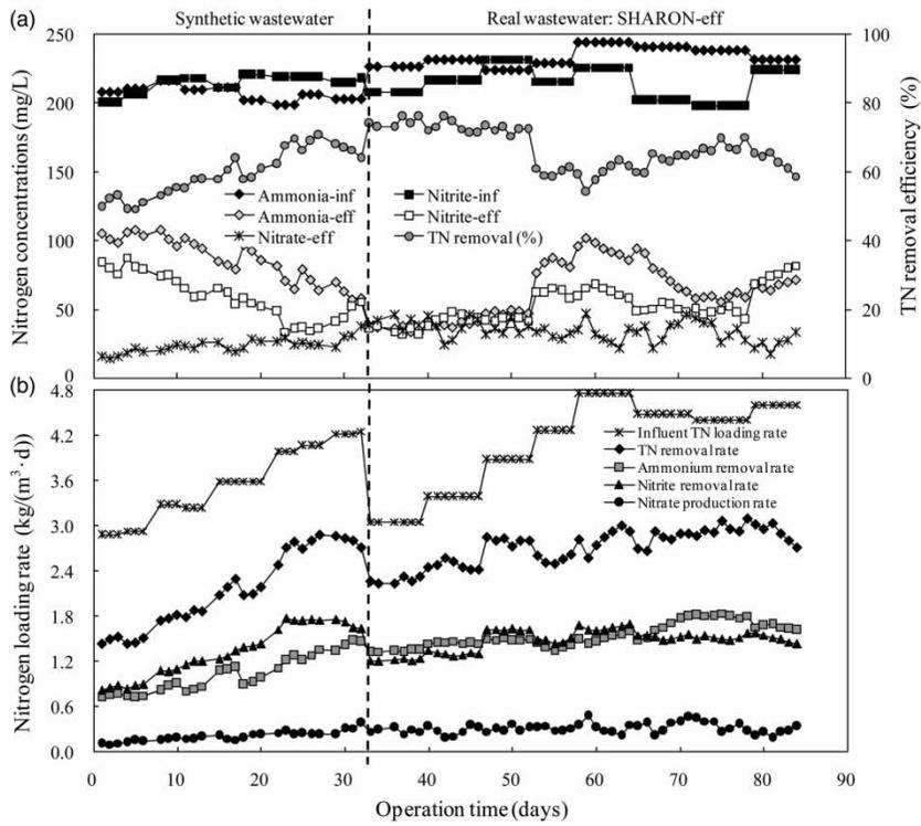
**Figure 2** (a) Concentrations of nitrogen compounds in the conventional ANAMMOX system treating synthetic and real wastewater. (b) Removal and production rates of nitrogen compounds in ANAMMOX process treating synthetic and real wastewater.
