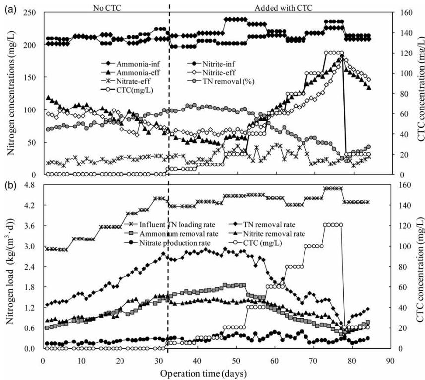
**Figure 3** (a) Concentrations of nitrogen compounds during the conventional ANAMMOX process under different CTC concentrations. (b) Removal and production rates of nitrogen compounds during the conventional ANAMMOX process under different CTC concentrations.
