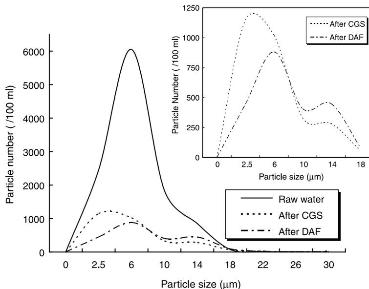
**Figure 5** Comparison of particle size distribution between sedimentation and flotation
