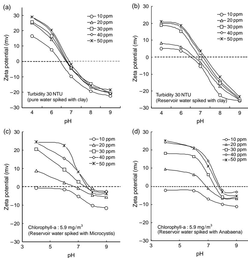
**Figure 2** Variations of zeta potential for two types of particles depending on coagulant dosages
