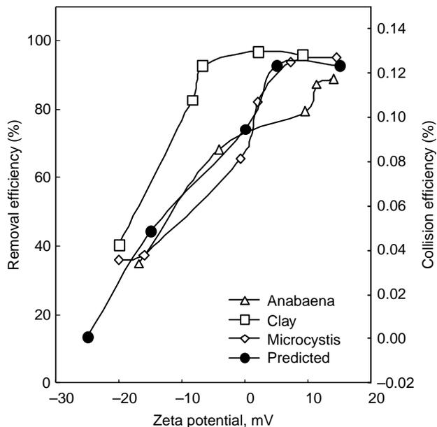
**Figure 7** Comparison of collision efficiency and removal efficiency in terms of zeta potential
