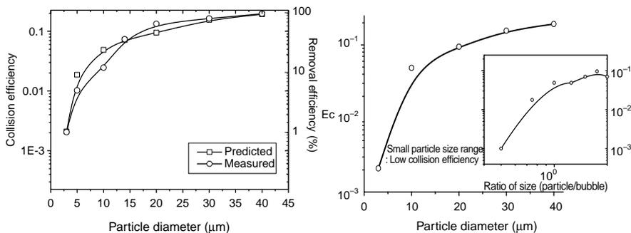
**Figure 8** Comparison of collision and removal efficiency in terms of particle diameter
