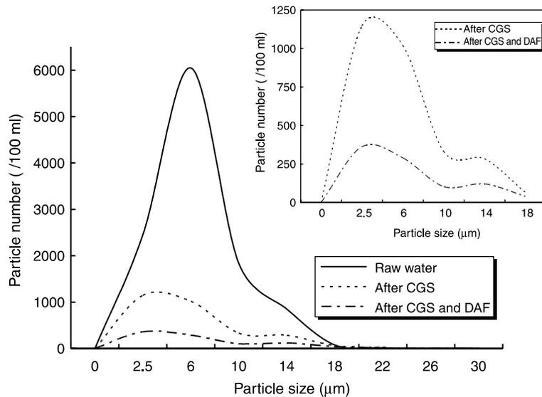
**Figure 6** Change of particle size distribution by flotation after sedimentation
