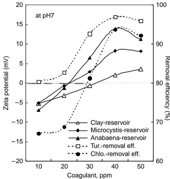
**Figure 3** Variation of removal efficiency and zeta potential depending on coagulant dosage
