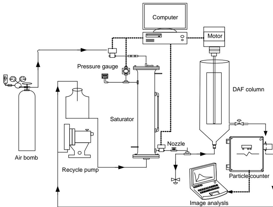
**Figure 1** The schematic diagram of DAF apparatus used in this experiment
