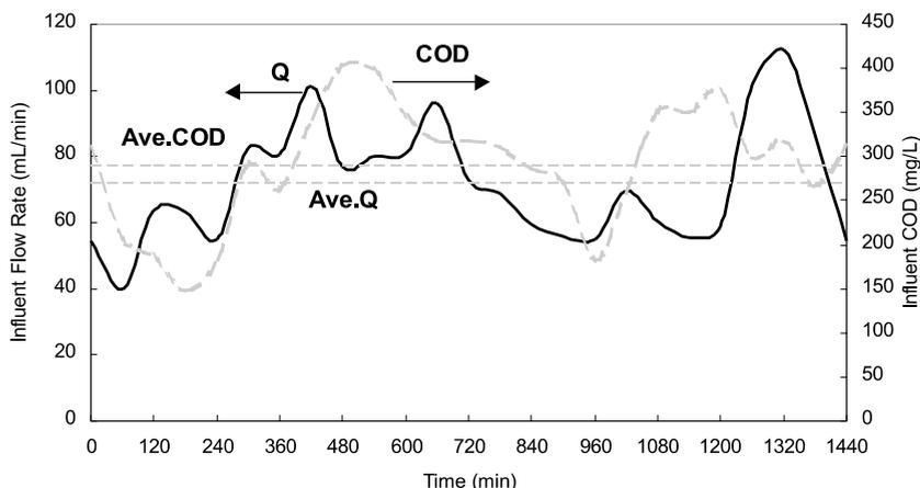
**Figure 2** Simulated dynamic influent conditions of continuous-flow SBR with varied  $F/M$  loadings
