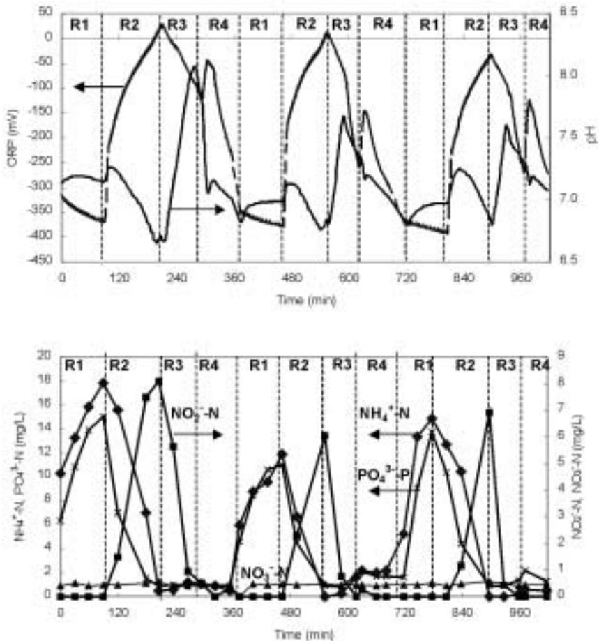
**Figure 5** Variations of water quality and monitoring parameters under ANN real-time controlled system.
