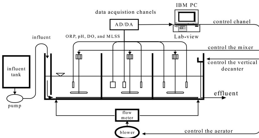
**Figure 1** Schematic diagram of continuous-flow SBR with monitoring and control system
