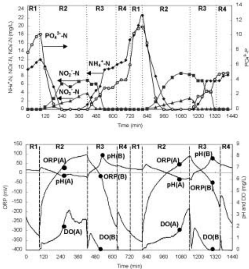
\*R1: Anaerobic phase; R2: Aerobic phase; R3: Anoxic phase; R4: Reaeration, Settling, and Discharge phases
