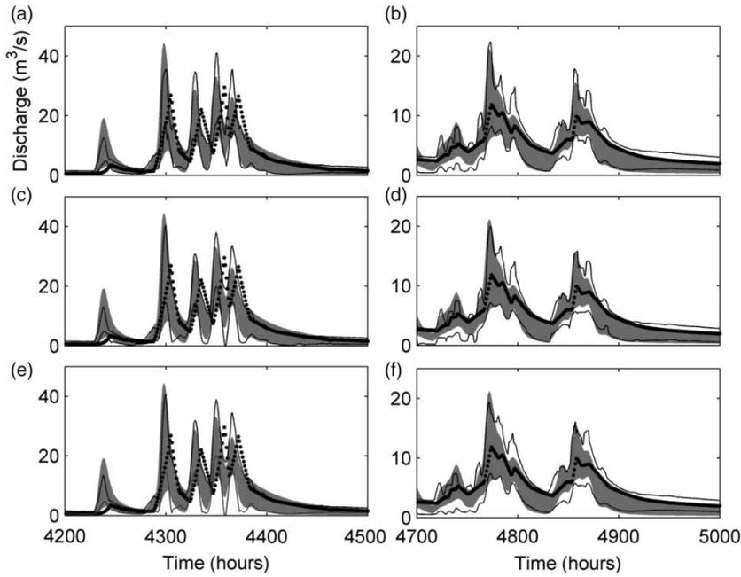
**Figure 4** | Hydrograph of 90% prediction bounds estimated by GLUE and machine learning methods for the Brue catchment in parts of the verification period. The black dots indicate the observed discharges and the dark grey shaded area – the prediction uncertainty that results from GLUE. The black lines denote the prediction uncertainty estimated by neural networks ((a) and (b)), model trees ((c) and (d)) and locally weighted regression ((e) and (f)).
