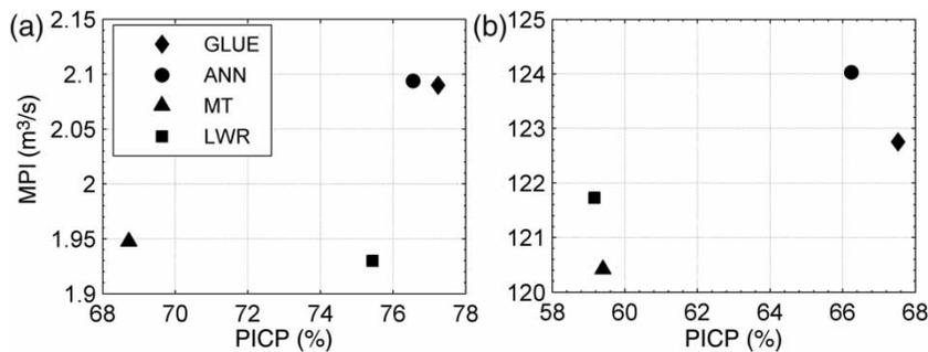
**Figure 6** | A comparison of statistics of uncertainty (PICP and MPI) estimated with GLUE, neural networks (ANN), model trees (MT), and locally weighted regression (LWR) in the verification period. (a) Brue catchment; (b) Bagmati catchment.
