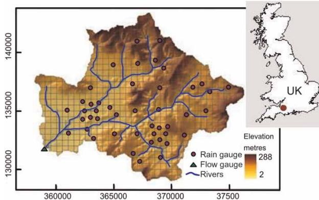
**Figure 2** | The Brue catchment showing dense rain gauges network (reproduced from Shrestha & Solomatine (2008) with permission from the International Association for Hydraulic Research). The horizontal and vertical axes refer to the easting and northing in British national grid reference co-ordinates. Circles denote the rainfall stations and triangles denote the discharge gauging stations. The location of the Brue catchment (solid circle) in the map of UK is shown in the inset.
