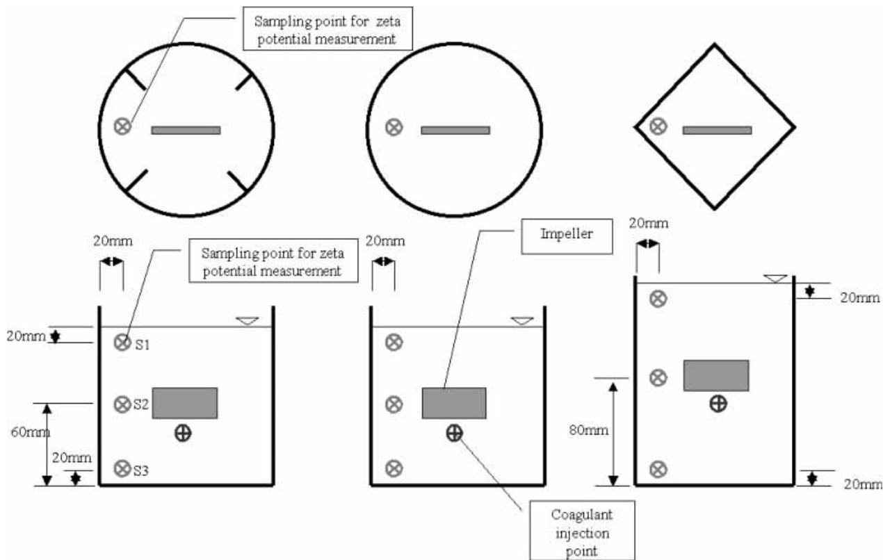
**Figure 2** | Schematic for zeta potential measurement and coagulant dose.
