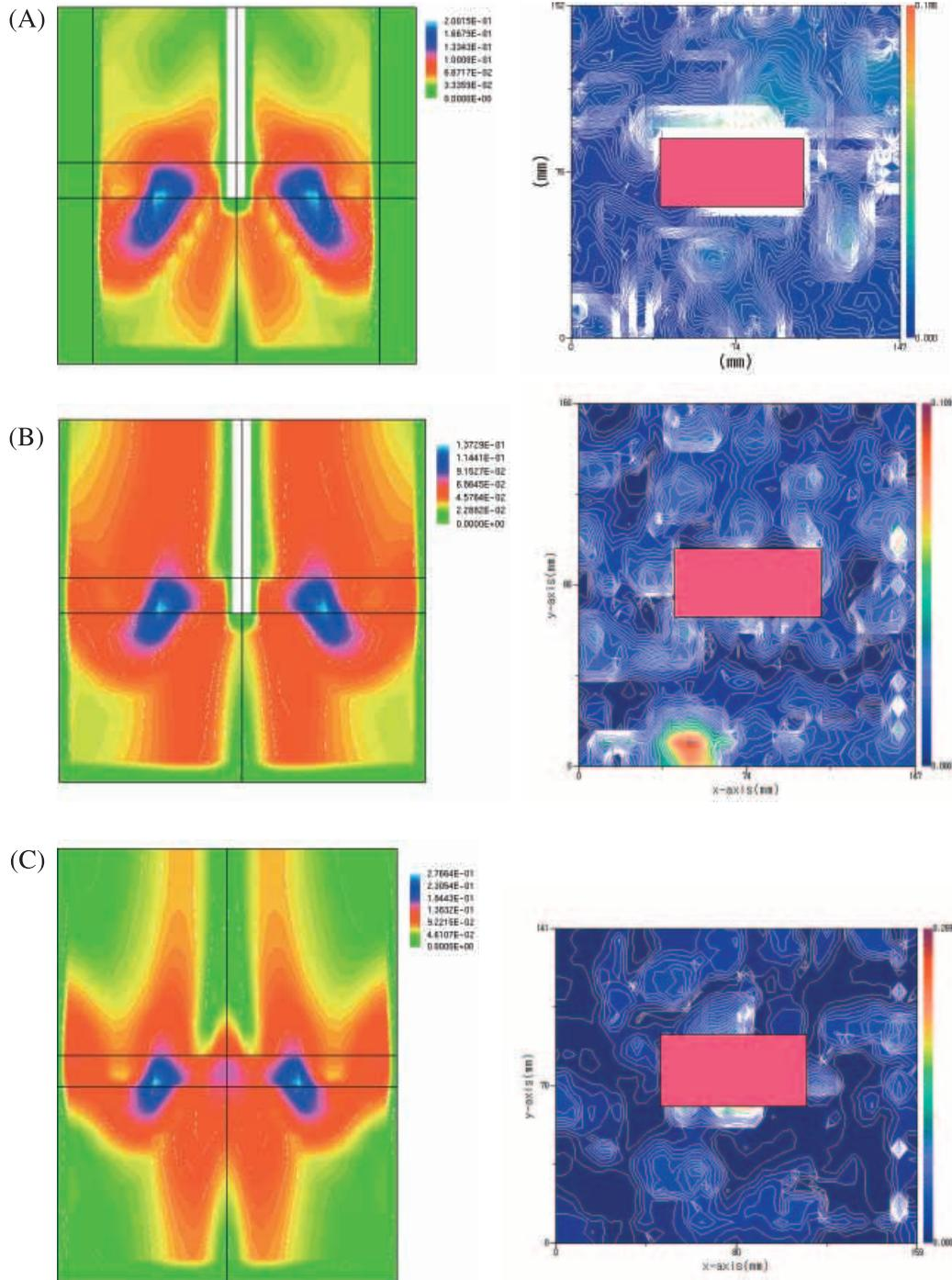
**Figure 6** | Contour of absolute value of velocity from results of CFD simulation (left column) and PIV analysis (right column): (A) circular baffled jar, (B) circular jar without baffles, (C) Hudson jar.
