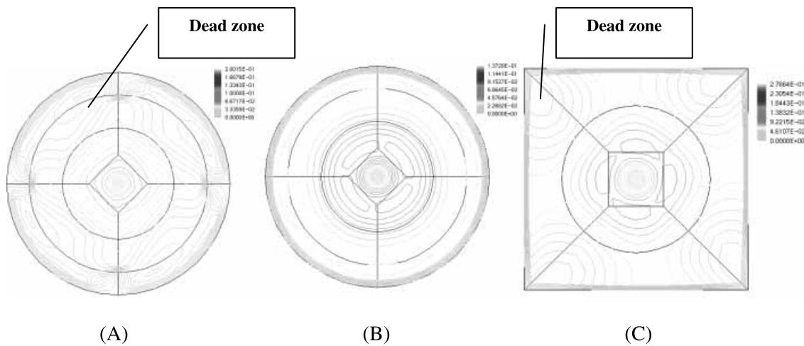
**Figure 7** | Formation of dead zones from the results of CFD simulation: (A) circular baffled jar, (B) circular jar without baffles, (C) Hudson jar.
