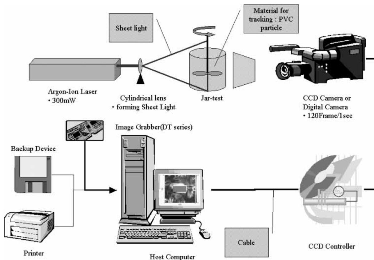
Figure 3 | Schematic of the PIV system used in this study.
