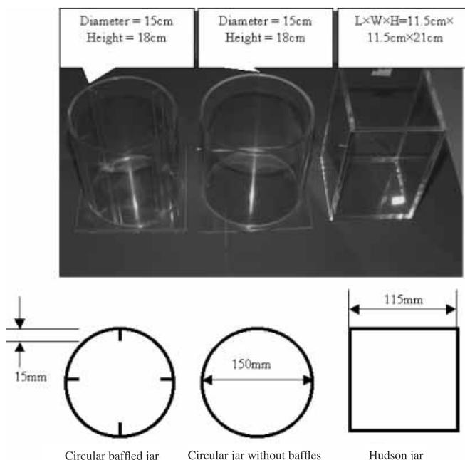
**Figure 1** | Three different types of jar used in the wet tests.
