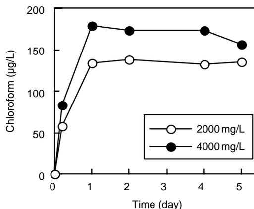
Figure 9 | Chloroform produced by chlorine dioxide.
