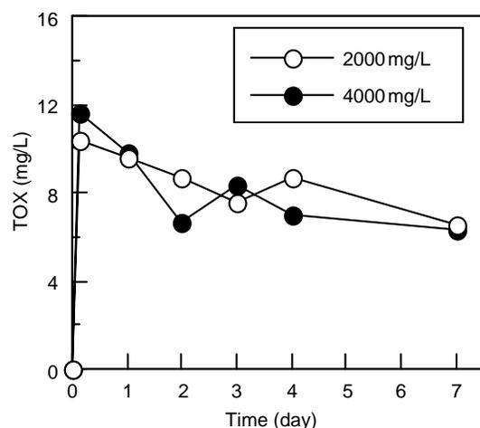
Figure 8 | TOX produced by chlorine dioxide.
