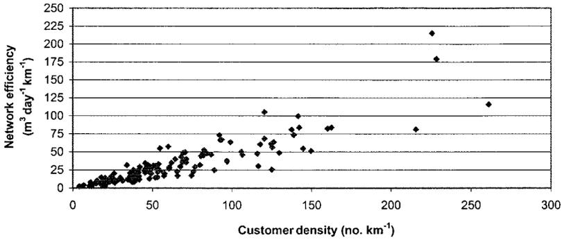
**Figure 3** Relation between customers density and network efficiency [Marques, 1999, (Data: APDA, 1997)]
