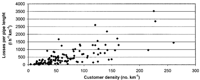
**Figure 5** Relation between network losses and customers density [Marques, 1999, (Data: APDA, 1997)]
