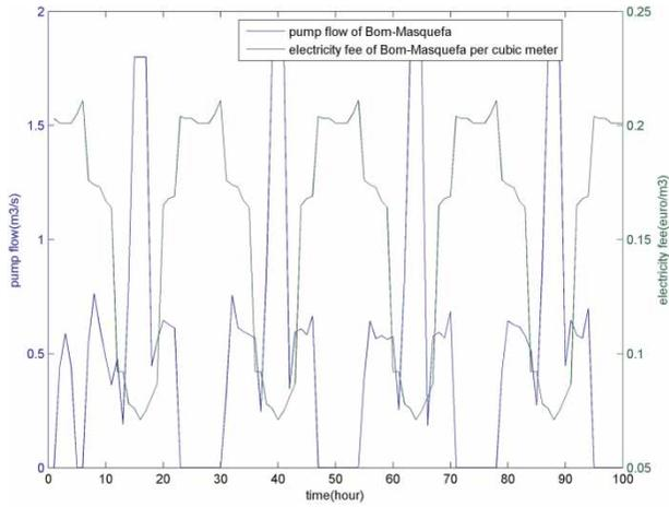
**Figure 8** | Pump flow with electricity price.
