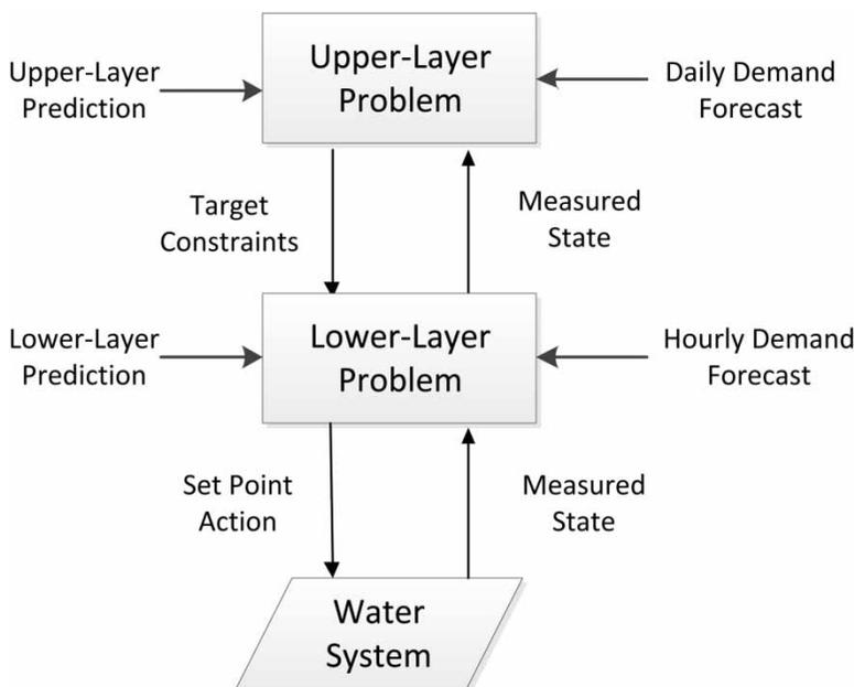
Figure 1 | Temporal hierarchy multi-layer MPC.
