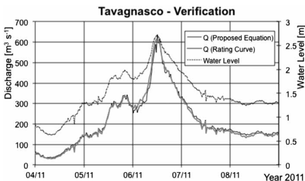
Figure 10 | A detail of the verification for the high flows observed in the period 4–9 November 2011. Comparison of the discharge estimates based on the steady-flow rating curve available at Tavagnasco gauging station on the Dora Baltea in Italy and the corresponding values estimated on the basis of the proposed approach, demonstrating a noticeable agreement.
