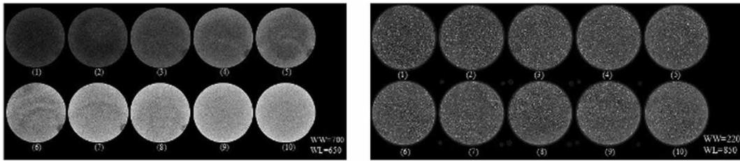
Figure 3 | Silica sand (left) and Yamazuna sand (right) CT images under initial conditions.
