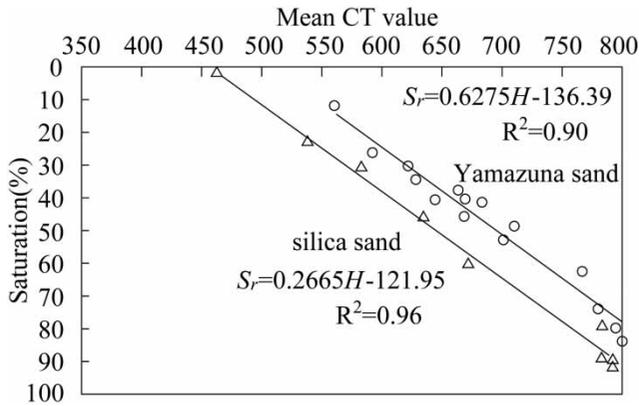
Figure 4 | The fitted linear of mean CT values vs. saturation.
