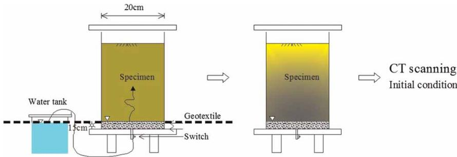
Figure 1 | Schematic diagram of apparatus.
