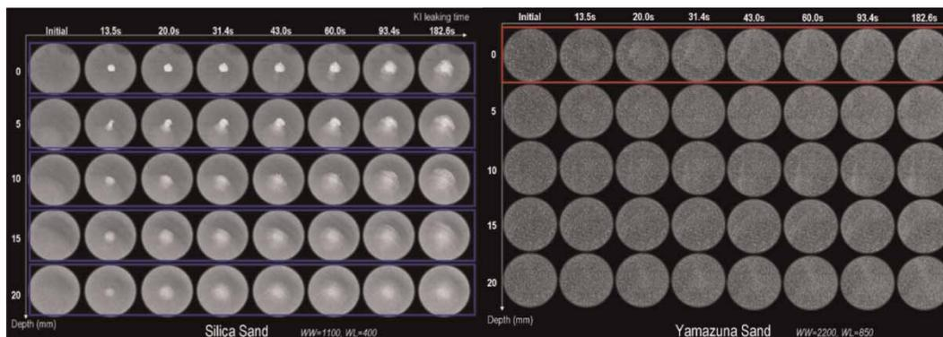
Figure 5 | CT scanning image after contaminant injection (only top five layers).
