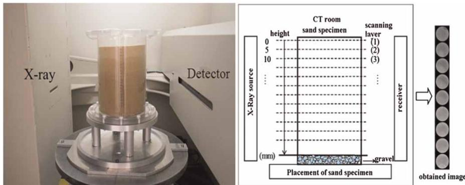
Figure 2 | The photograph and scheme of the specimen in CT room.
