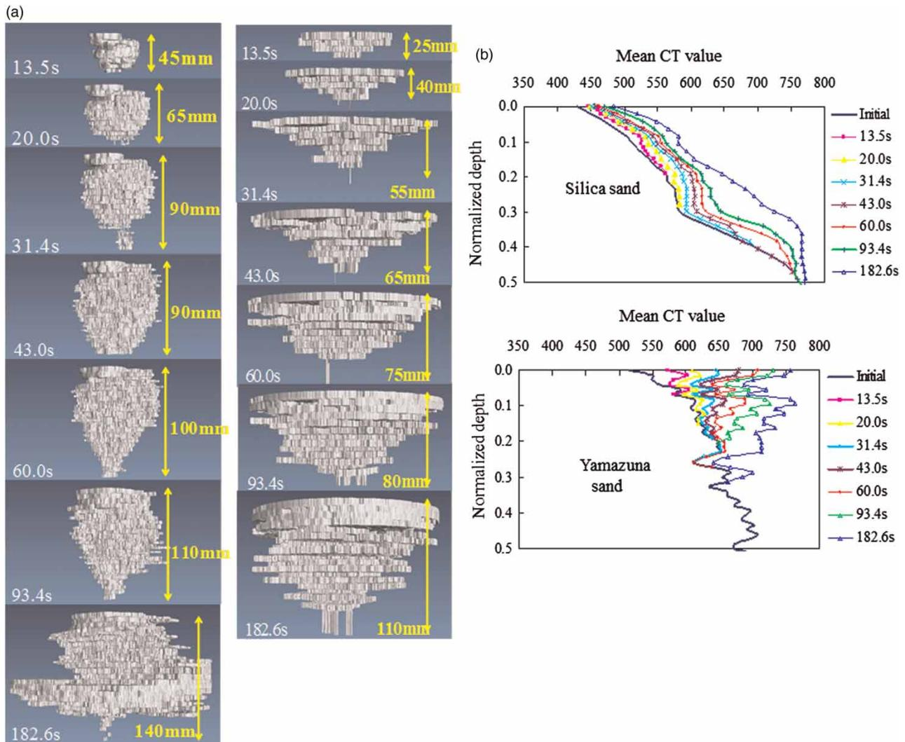
**Figure 6** | (a) 3D-reconstruction images by VGStudio generated from individual CT scanner slice image data. Silica sand (left) Yamazuna sand (right); (b) The migration results of KI with depths and time in sand specimens.
