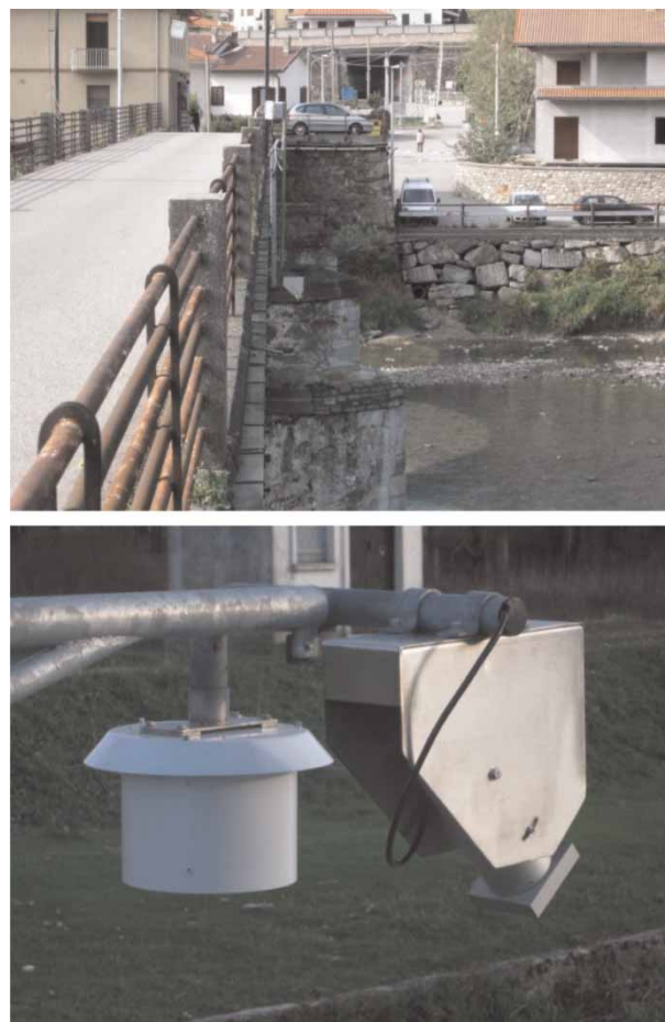
Figure 3 | The cross-section of Tavagnasco on the Dora Baltea in Italy where the sensor was installed (top) and a detail of water level and surface velocity sensors (bottom) used for flow measurements.
