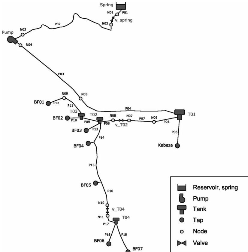
Figure 3 | The water distribution network of Mataba (Rwanda).
