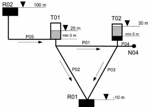
**Figure 9** | mLBC test case. Schematic representation of the WDN. Two emptying and filling interconnected tanks with different initial and minimum levels. The arrows indicate the positive sign of the water flow.
