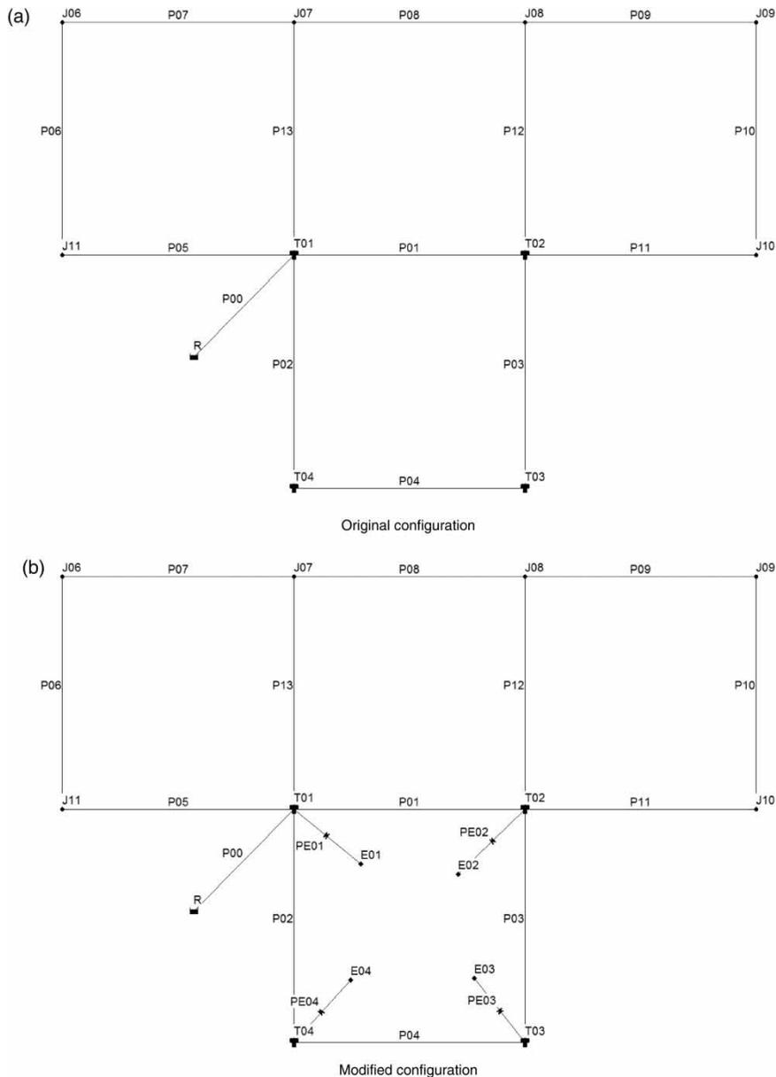
**Figure 6** | MLBC test case: schematic representation of the WDN.
