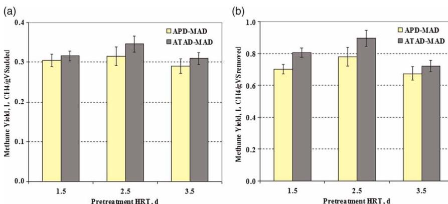
Figure 5 | (a and b) Methane yield for the MAD reactors.
