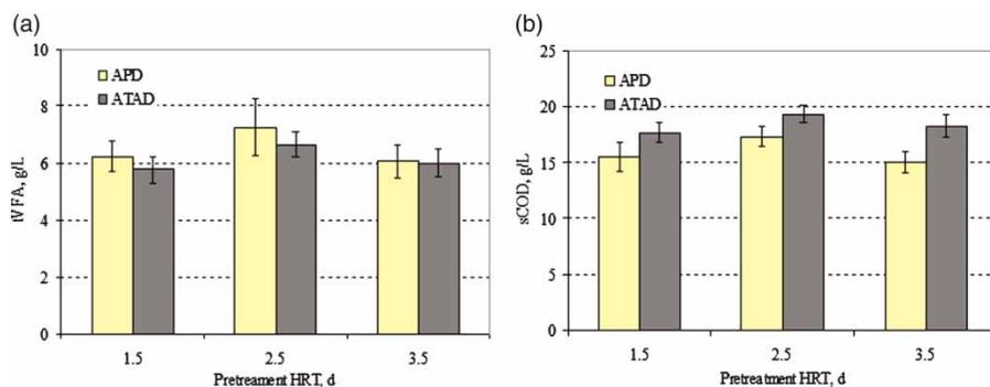
Figure 3 | (a and b) Total VFA and sCOD levels for APD and ATAD at different HRTs.
