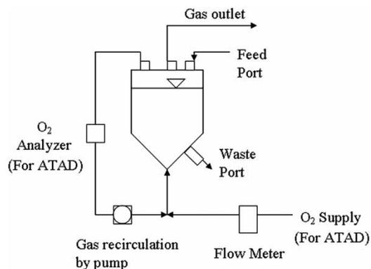
Figure 1 | Set-up for the ATAD reactor.
