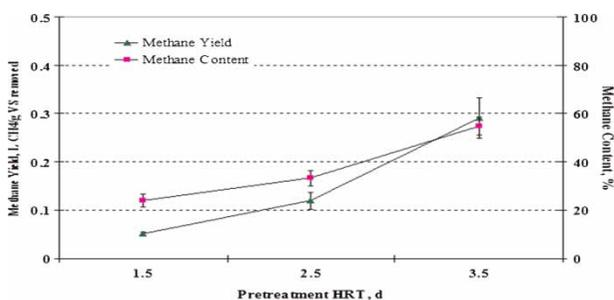
Figure 4 | Methane yield and methane content for APD for different HRTs.
